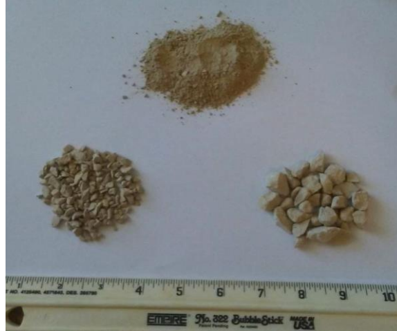
Figure 2. Fly ash and granular pellets. Top raw fly ash, lower right, 0.25 to 0.50 inch pellets, lower left, 0.08 to 0.5 inch pellets.
