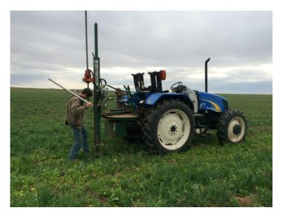
Figure 2. Soil coring device used in one of the study fields
