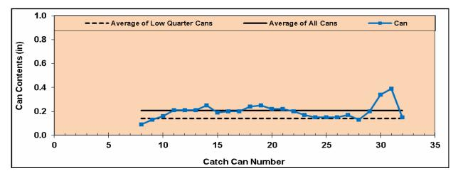
Figure 2: Example of acceptable uniformity in tested Ogallala irrigation system
