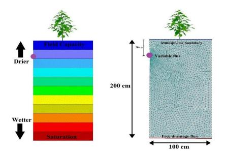
Figure 1. Physical layout, initial, and boundary conditions of the simulated
