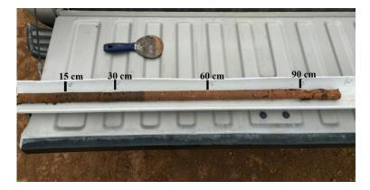
Figure 3. soil core and sub-cores lengths
