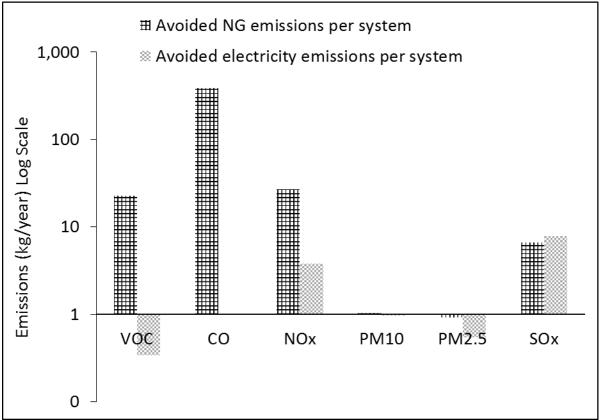
Figure 12. Log scale of primary pollutants for average individual system (electric and gas) tested – not including greenhouse gases
