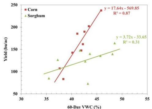
**Figure 5:** the relationship between yield observed in the south rows and the volumetric water content (VWC) measure within the south rows at 6 inches below the soil surface. The VWC data were averaged over a 2-month period which was Jul 9 to Sep 7 for corn and Jul 18 to Sep 15 for sorghum.
