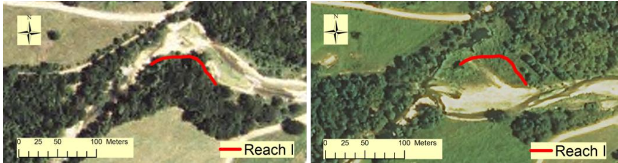
Figure 1.21. Streambank erosion at reach I on the Barren Fork Creek from National Agricultural Imagery Program aerial 2003 (left) to 2013 (right) images. The red line is the location of the reach in 2003.
