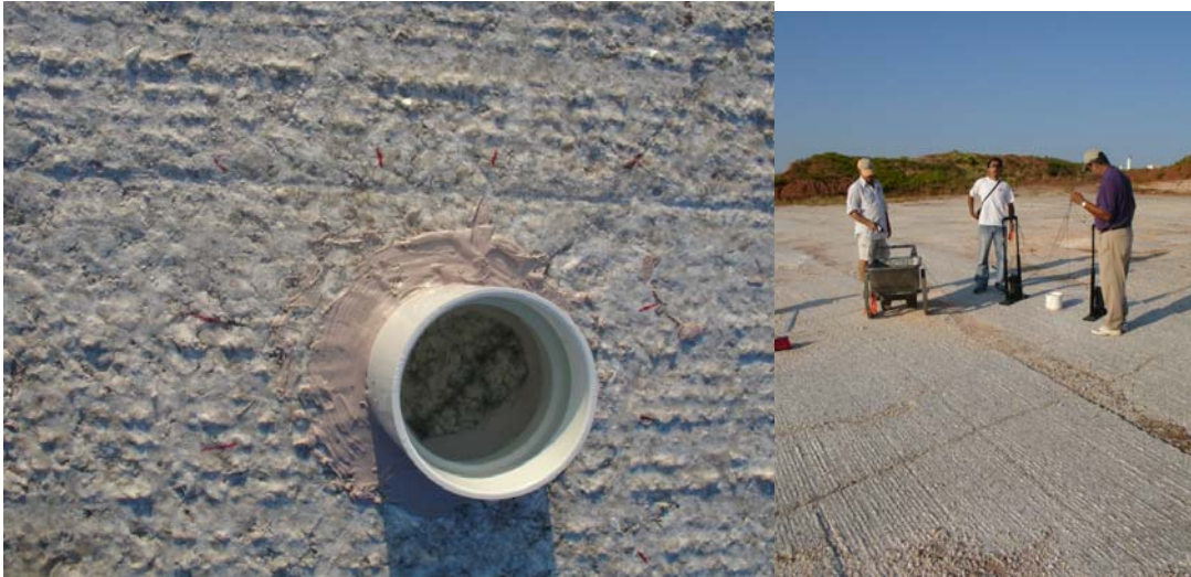
Figure 5. Six inch PVC coupler bonded to a NE-SW fracture (left) in preparation for infiltration experiment. The picture on the right shows the polarization experiment being conducted for dry and saturated fracture conditions.
