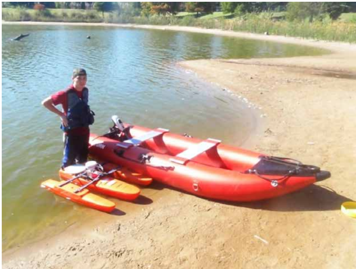
Figure 5: The Teledyne RDI Workhorse Rio Grande 600 kHz Acoustic Doppler Current Profiler (ADCP) with Hemisphere RTK-GPS and the inflatable “KaBoat”
