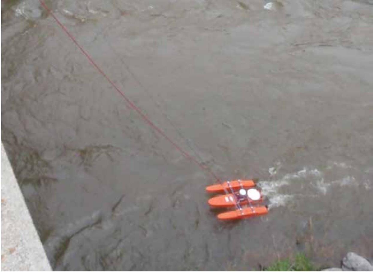
Figure 4: Teledyne RDI Workhorse Rio Grande 600 kHz Acoustic Doppler Current Profiler (ADCP) operating from a bridge.
