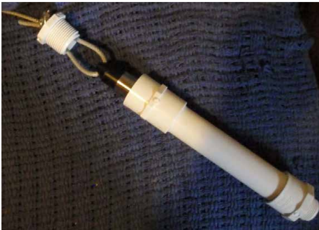
Figure 7: HOBO Water Level Logger with PVC housing.
