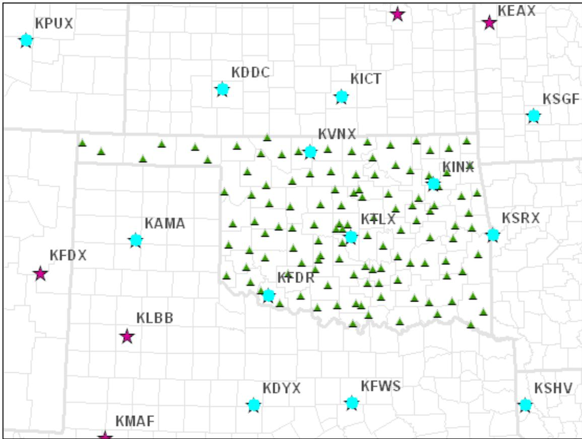
Figure 2: ScourCast observational network composed of 13 NWS Radars and 120 Oklahoma Mesonet Rain Gauges
