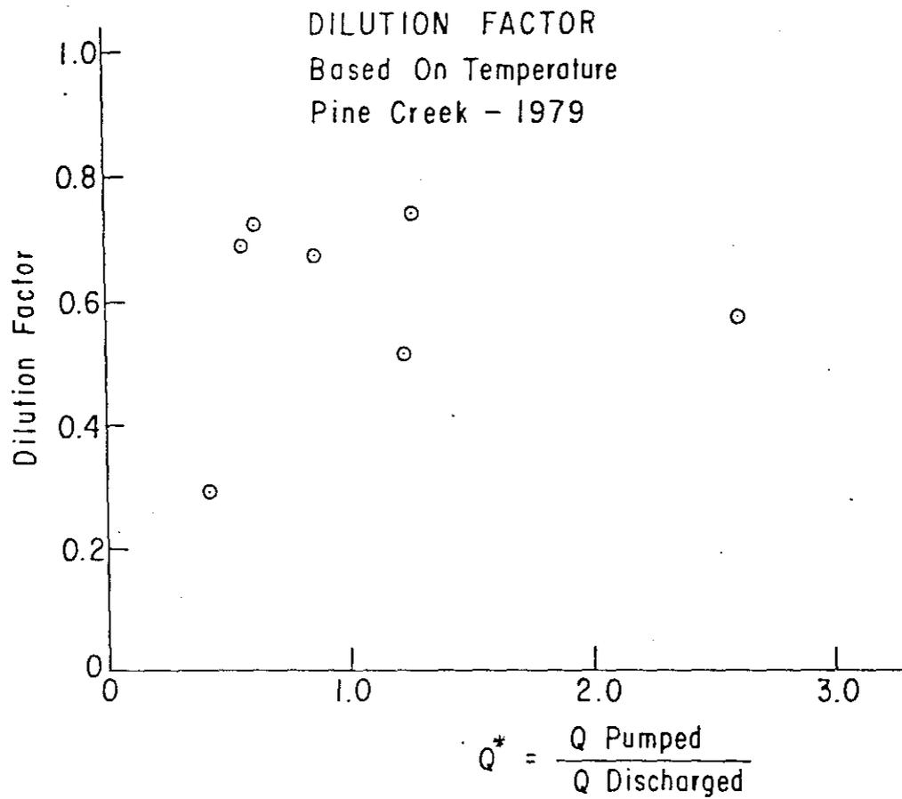
Figure 2-2. The Relationship of Dilution Factor (percent of surface water being released) to the Ratio of Pump Discharge to Discharge Rate.
