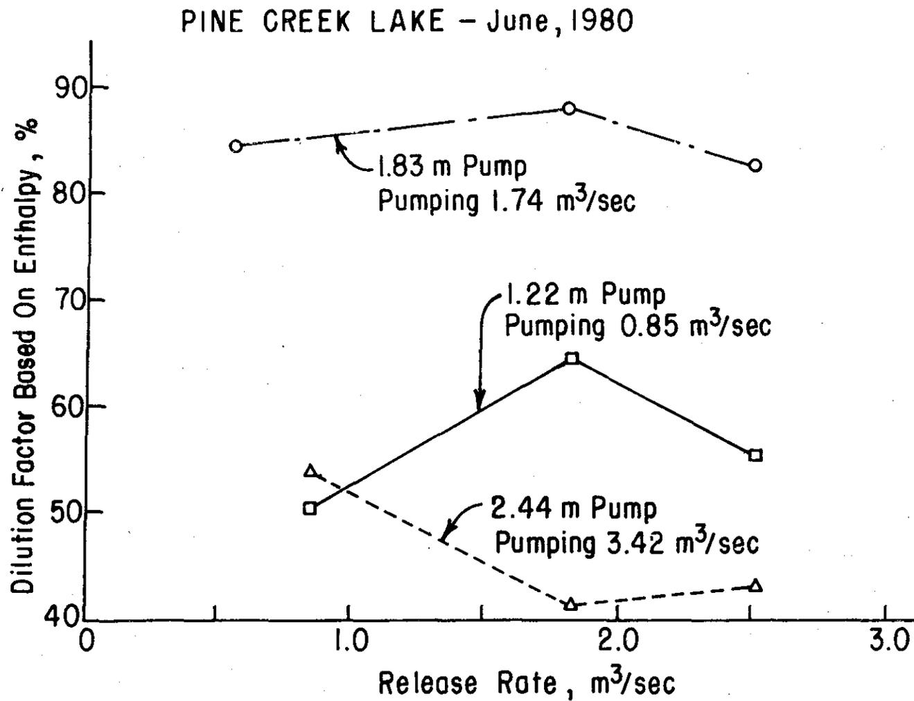
Figure 2-9. Dilution Factor Based on Enthalpy as a Function of Release Rate at Pine Creek on 26 June 1980
