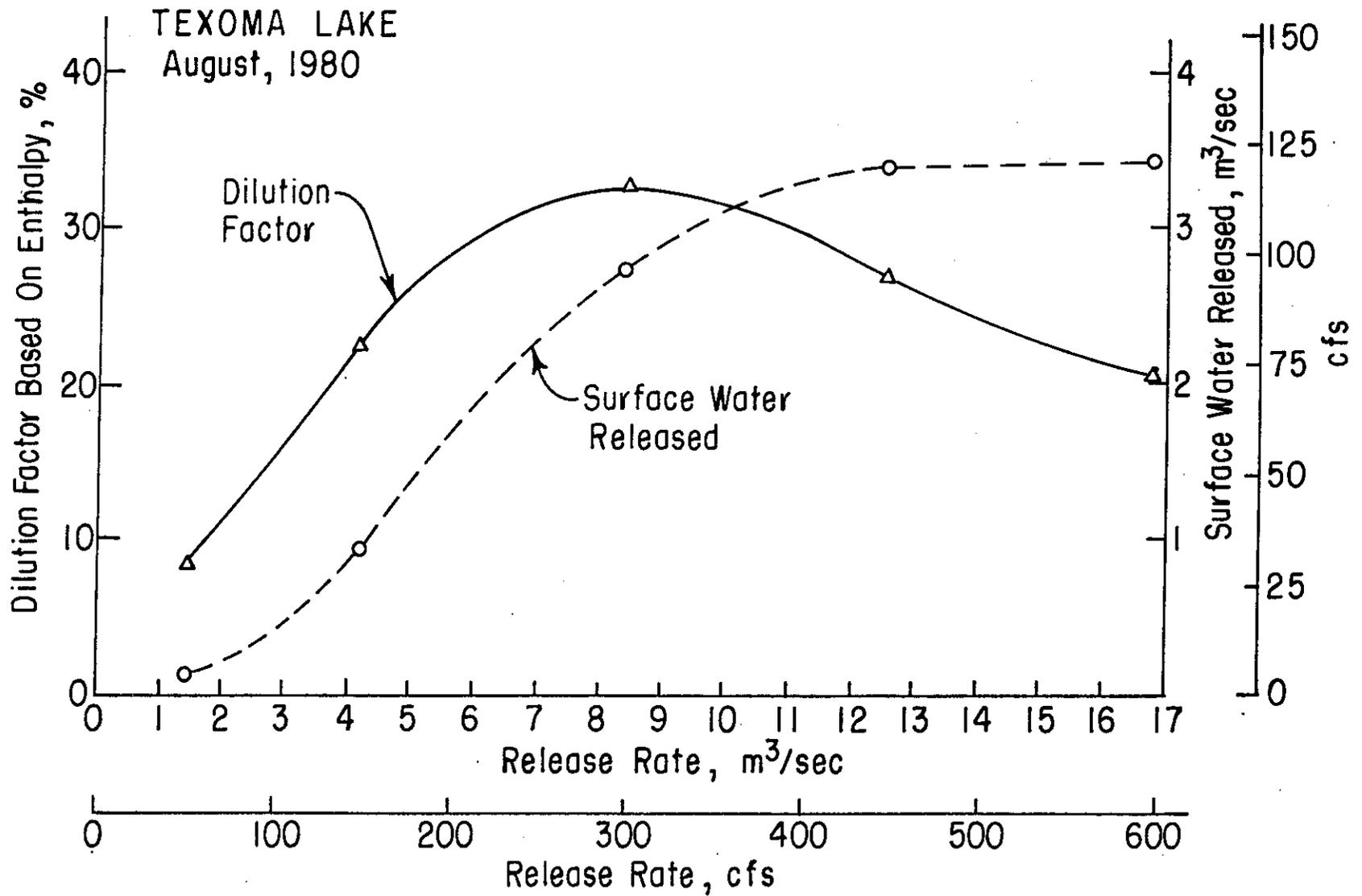
Figure 1-13. Dilution Factor and Surface Water Release Rate as a Function of Reservoir Release at Lake Texoma
