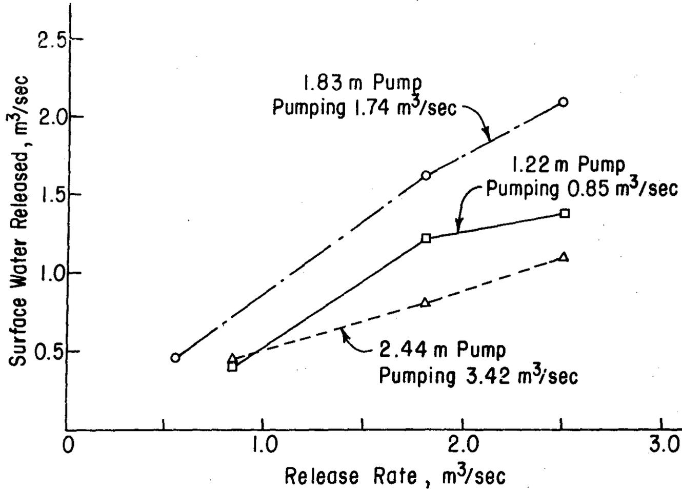
Figure 2-10. Surface Water Release Rate as a Function of Reservoir Release Rate at Pine Creek on 26 June 1980
