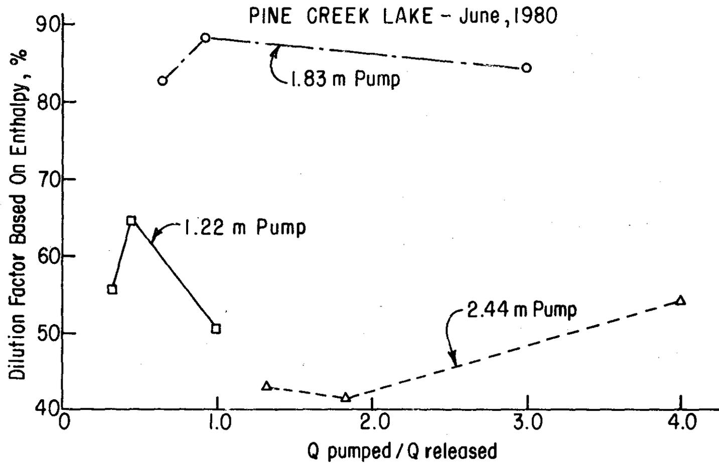
Figure 2-11. Dilution Factor Based on Enthalpy as a Function of the Ratio of Pumping to Release Rate at Pine Creek on 26 June 1980
