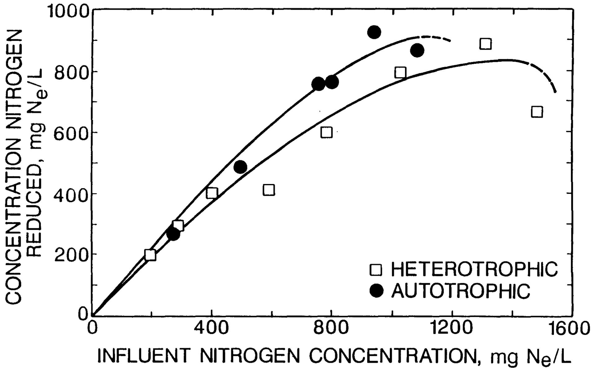
Figure 6. Influent nitrogen concentration limits on treatment efficiency in USB reactors operated at constant 6 hour HRT.
