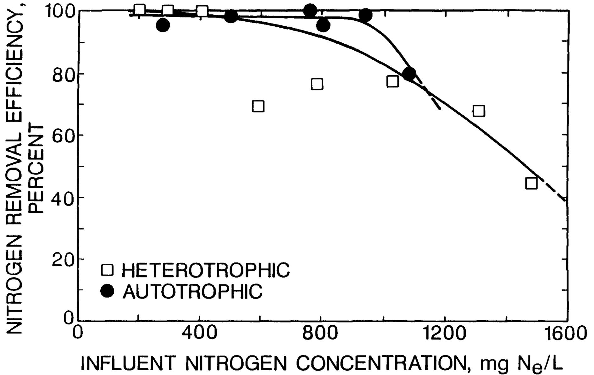
Figure 5. Treatment efficiency as a function of influent nitrogen concentration in USB reactors operated at constant 6 hour HRT.
