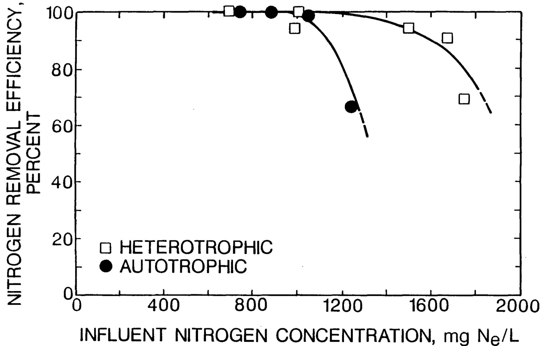
Figure 3. Treatment efficiency as a function of influent nitrogen concentration in AFEB reactors operated at constant 3.5 hour HRT.
