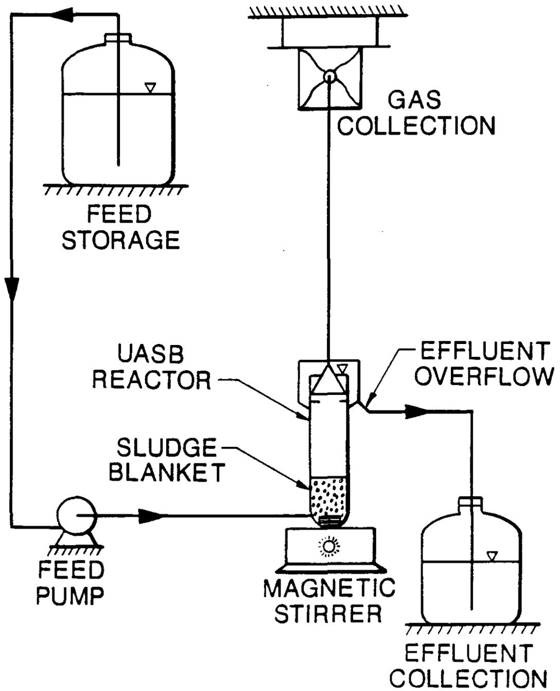
Figure 2. Schematic of the bench-scale experimental USB systems.
