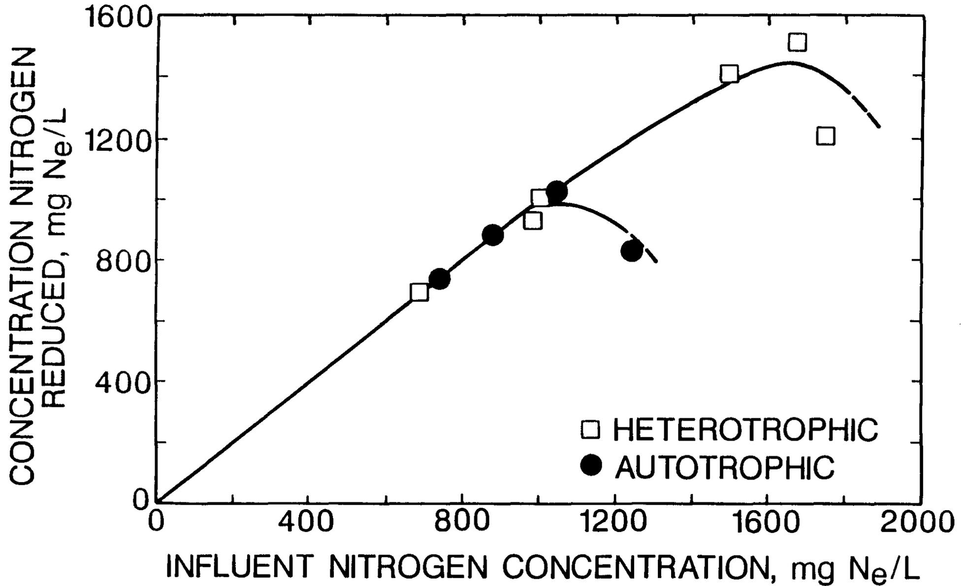
Figure 4. Influent nitrogen concentration limits on treatment efficiency in AFEB reactors operated at constant 3.5 hour HRT.
