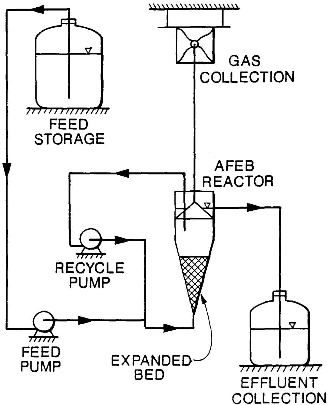
Figure 1. Schematic of the bench-scale experimental AFEB systems.
