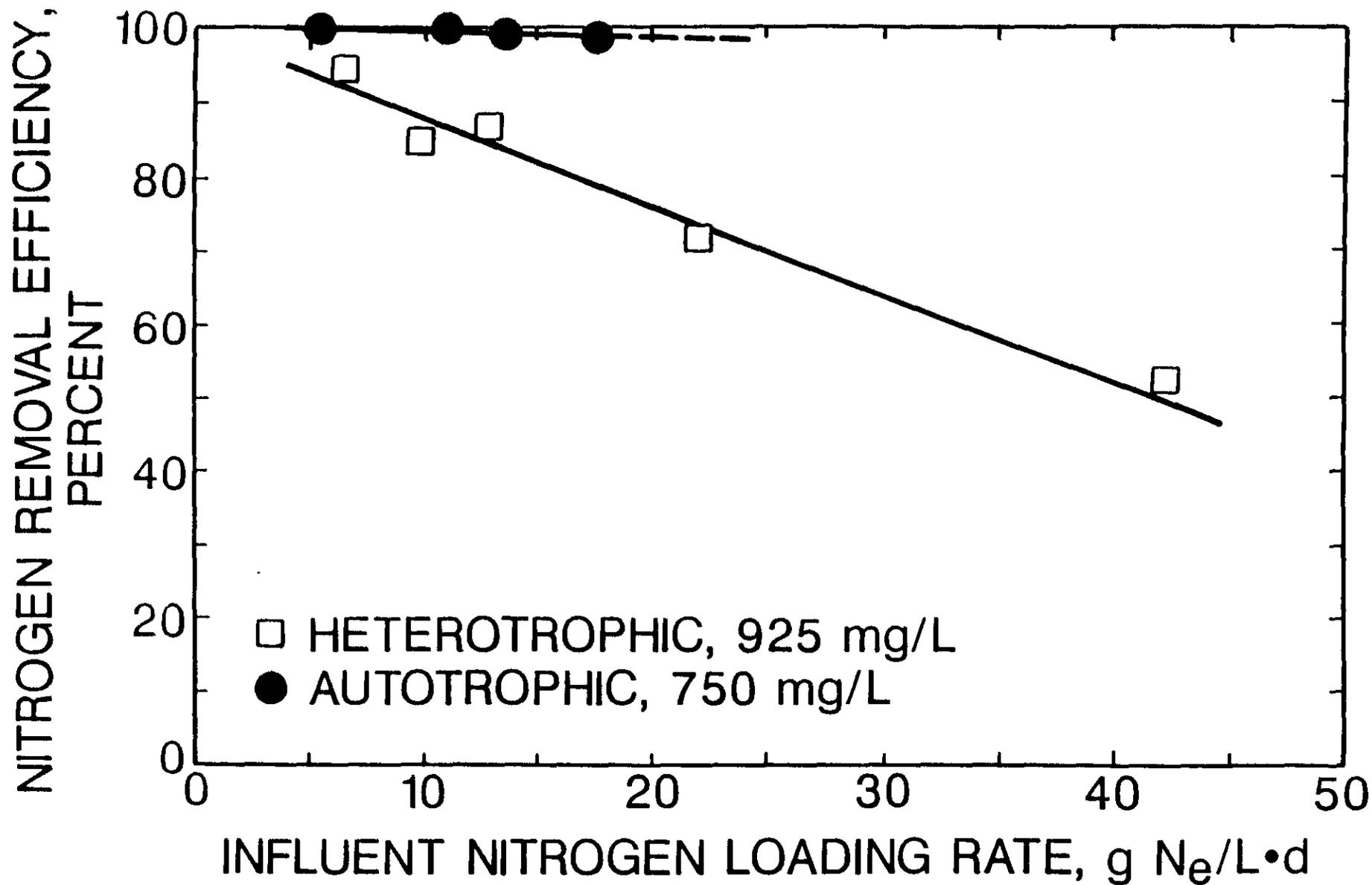
Figure 7. Treatment efficiency as a function of loading rate in AFEB reactors operated at constant feed concentrations (Heterotrophic = 925 mg Ne/L, Autotrophic = 750 mg Ne/L).
