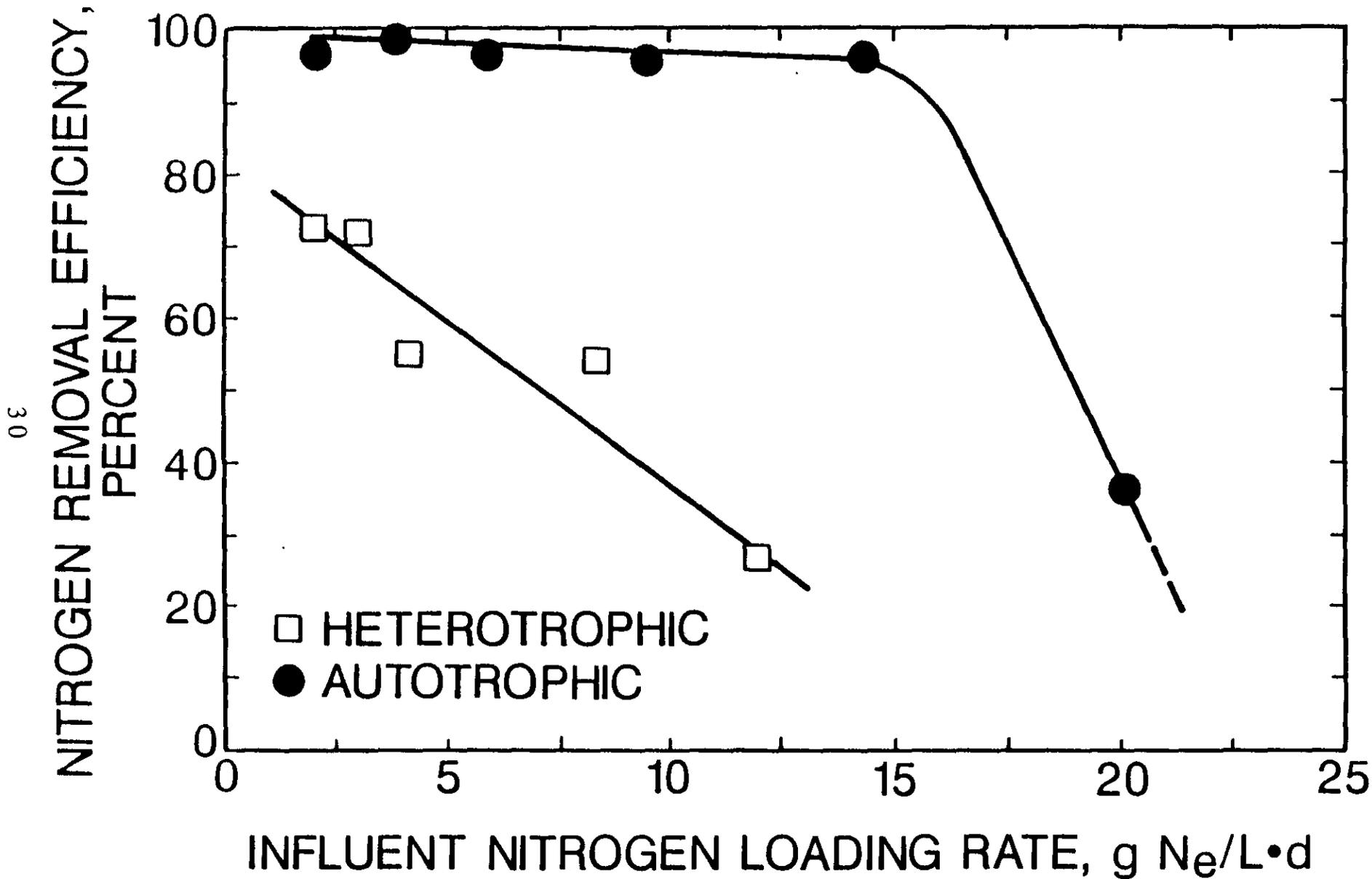
Figure 8. Treatment efficiency as a function of loading rate in USB reactors operated at constant feed concentration of 500 mg  $N_e/L$ .
