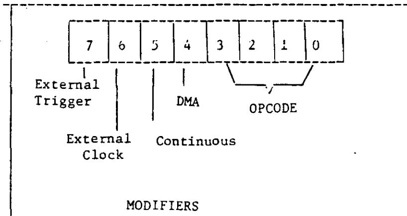
Figure 5. Command Register Bit Functions
