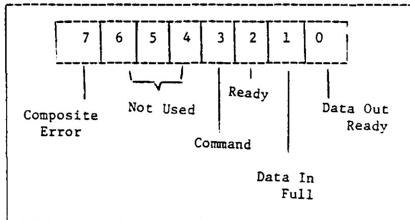
Figure 7. Status Register Bit Functions
