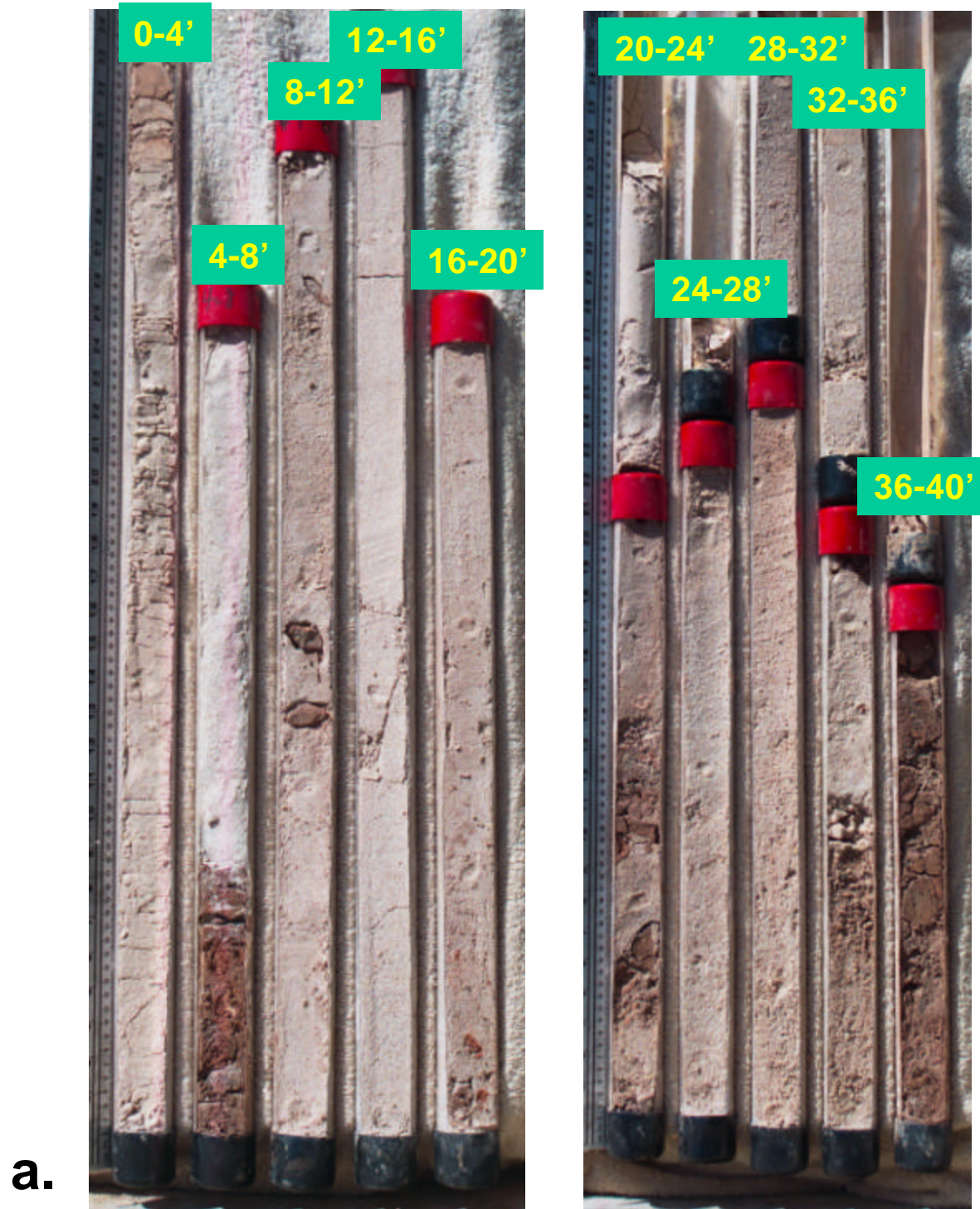
Figs. 8a, b (facing page) – Cores from Well #1 showing sand / mud layers and mud clasts. Each core segment is 4' in length though compaction of the sediment and loss of some materials (failure of core catcher?) always results in core length segments that are <4'.
