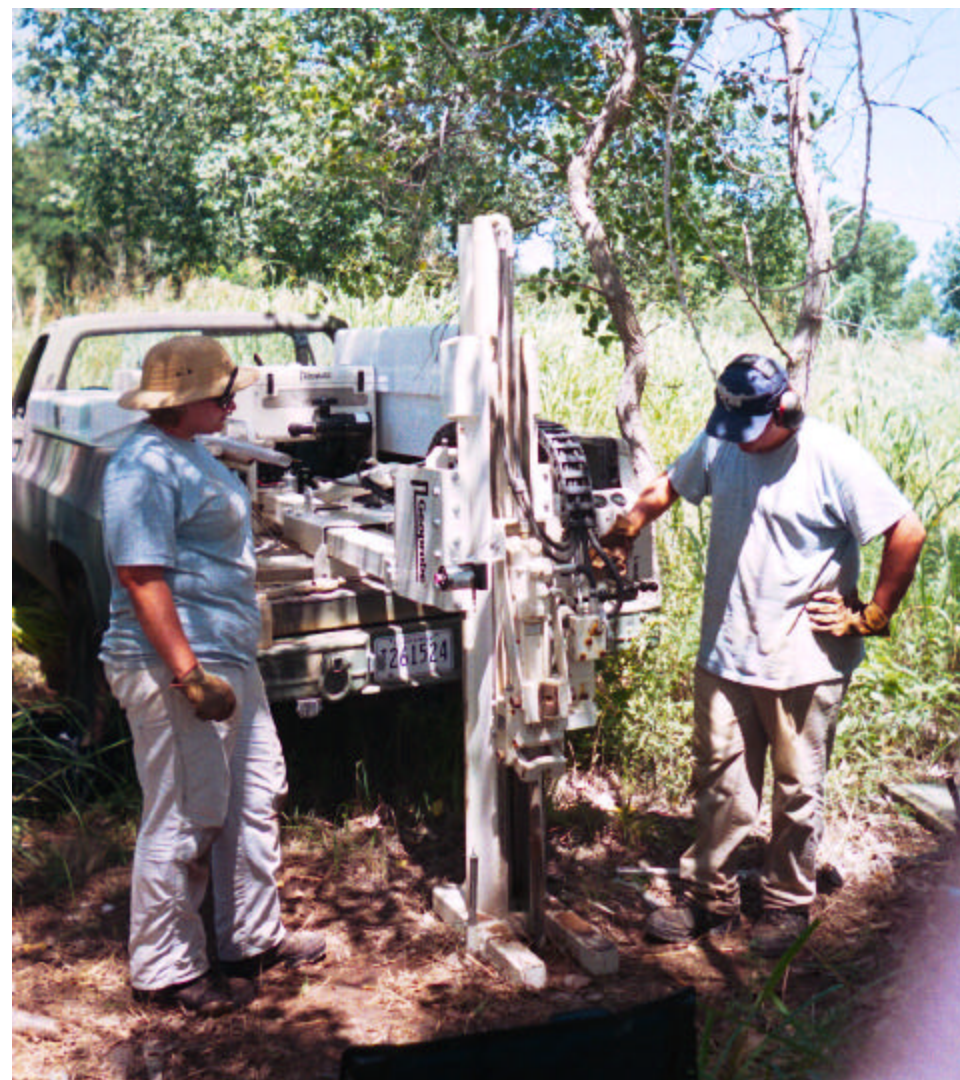
Fig. 3 – Kelli Collins and Tom Kropatsch collect conductivity data in the Canadian River floodplain.
