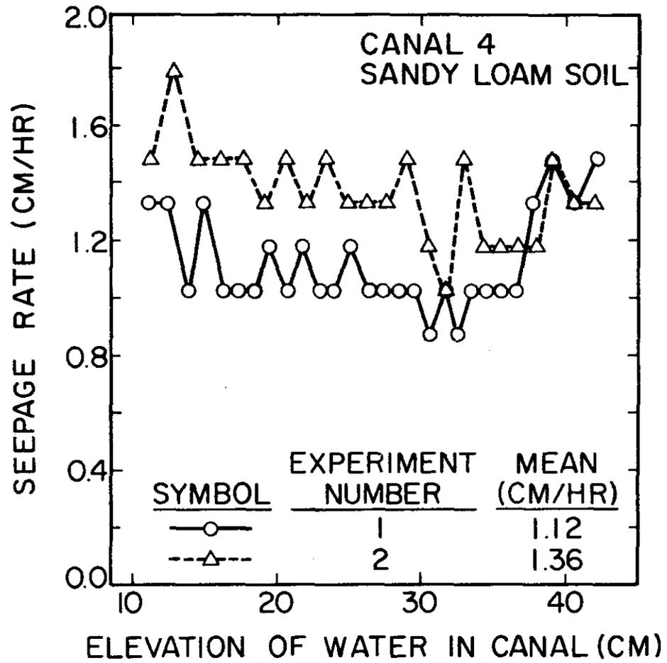
Figure 5. Seepage rate as a function of the elevation of water in the canal as measured by ponding.
