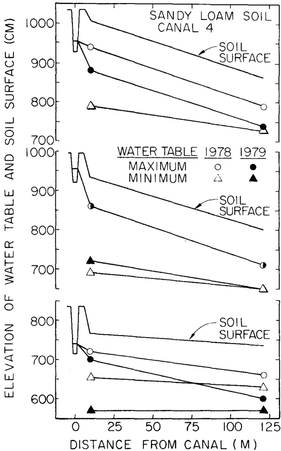
Figure 10. Minimum and maximum water table elevations in 1978 and 1979 for 3 sites approximately 140 m apart. This area was not irrigated.
