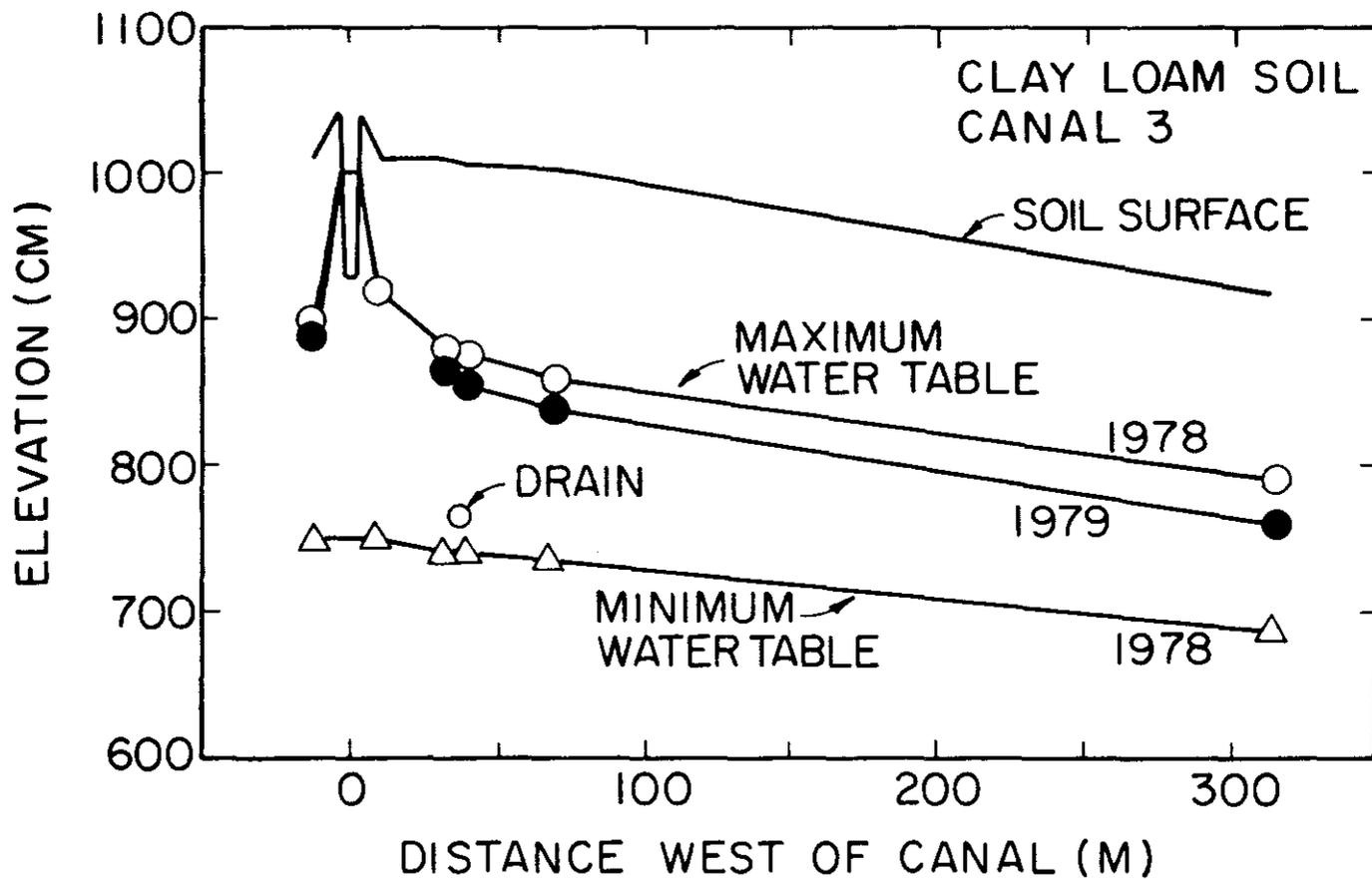
Figure 8. Minimum and maximum water table elevations in 1978 and 1979.
