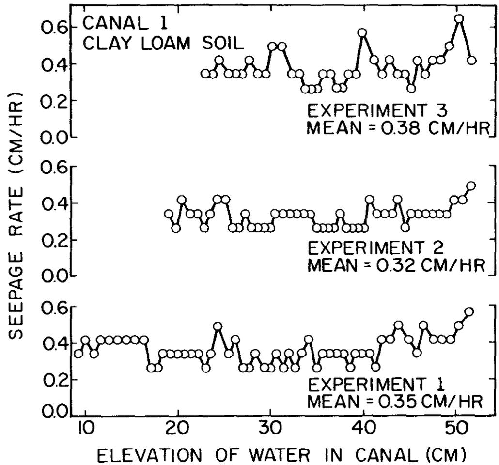
Figure 2. Seepage rate as a function of the elevation of water in the canal as measured by ponding.
