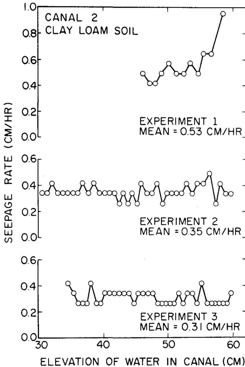
Figure 3. Seepage rate as a function of the elevation of water in the canal as measured by ponding.
