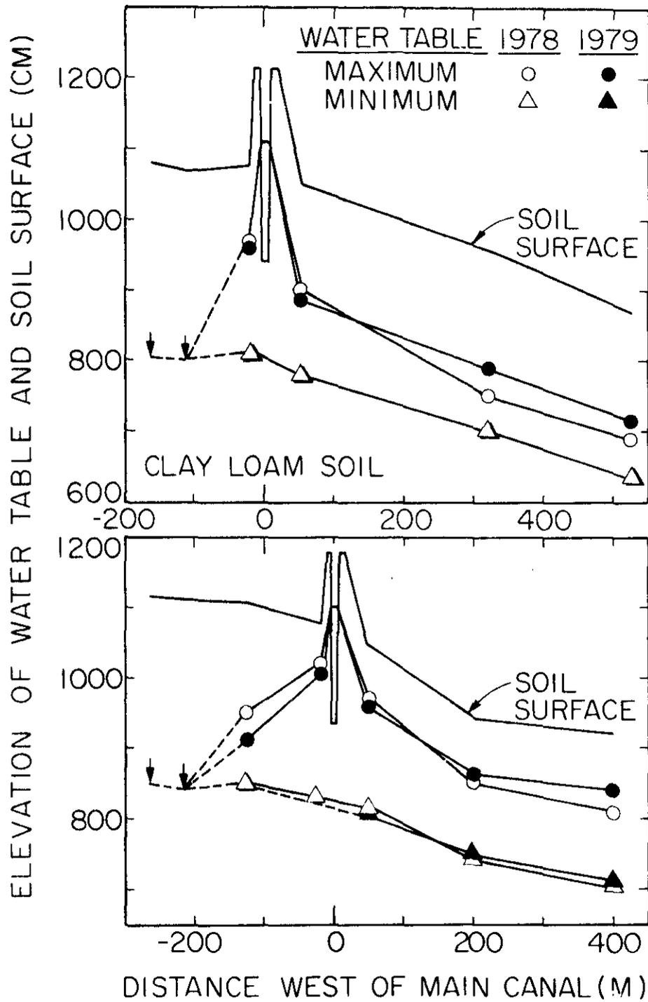
Figure 9. Minimum and maximum water table elevations in 1978 and 1979 for 2 sites 200 m apart. Dashed lines and arrows indicate water table was below deepest piezometer.
