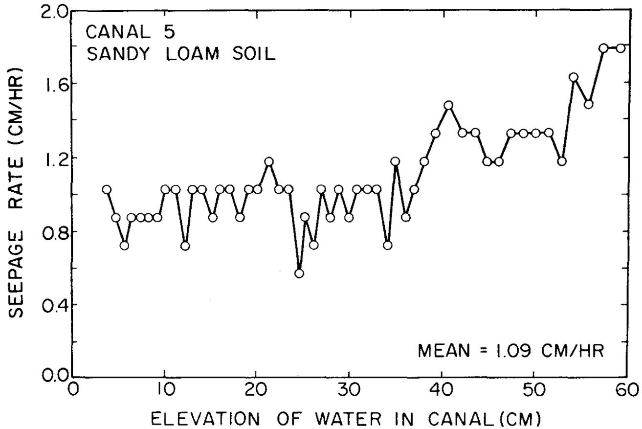
Figure 6. Seepage rate as a function of the elevation of water in the canal as measured by ponding.
