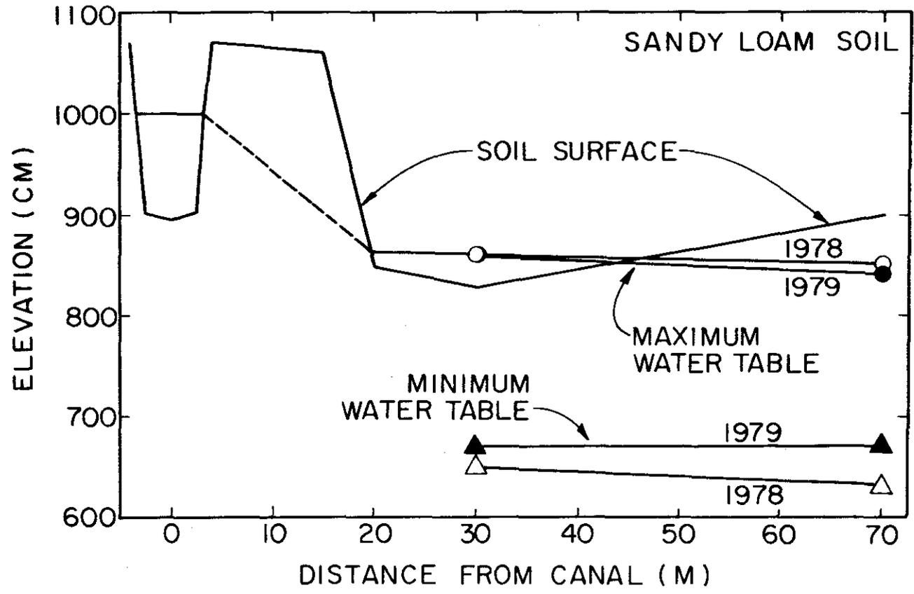
Figure 11. Minimum and maximum water table elevations in 1978 and 1979. This area was not irrigated.
