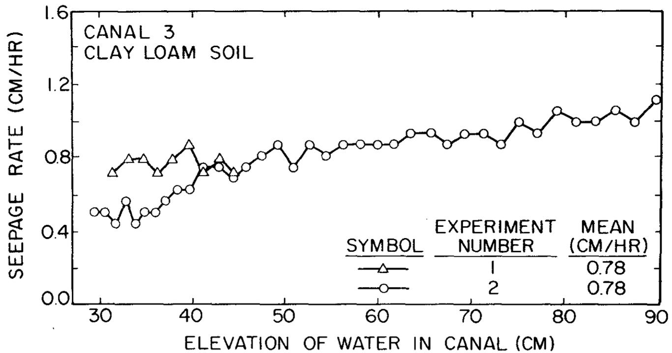
Figure 4. Seepage rate as a function of the elevation of water in the canal as measured by ponding.
