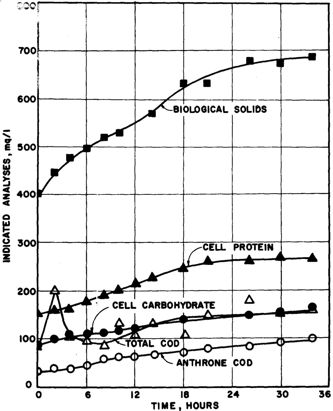
FIGURE 7. RESPONSE TO SHOCK LOAD;  $S_i$  1000→2000 mg/l AT  $\bar{t} = 12$  HOURS; ONCE THROUGH SYSTEM
