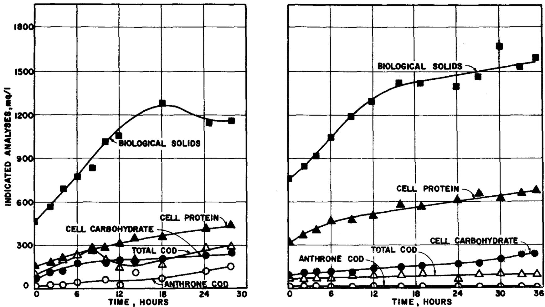
FIGURE 8. RESPONSE TO SHOCK LOAD;  $S_i$  1000  $\rightarrow$  3000 mg/l AT  $\bar{t} = 12$  HOURS;
