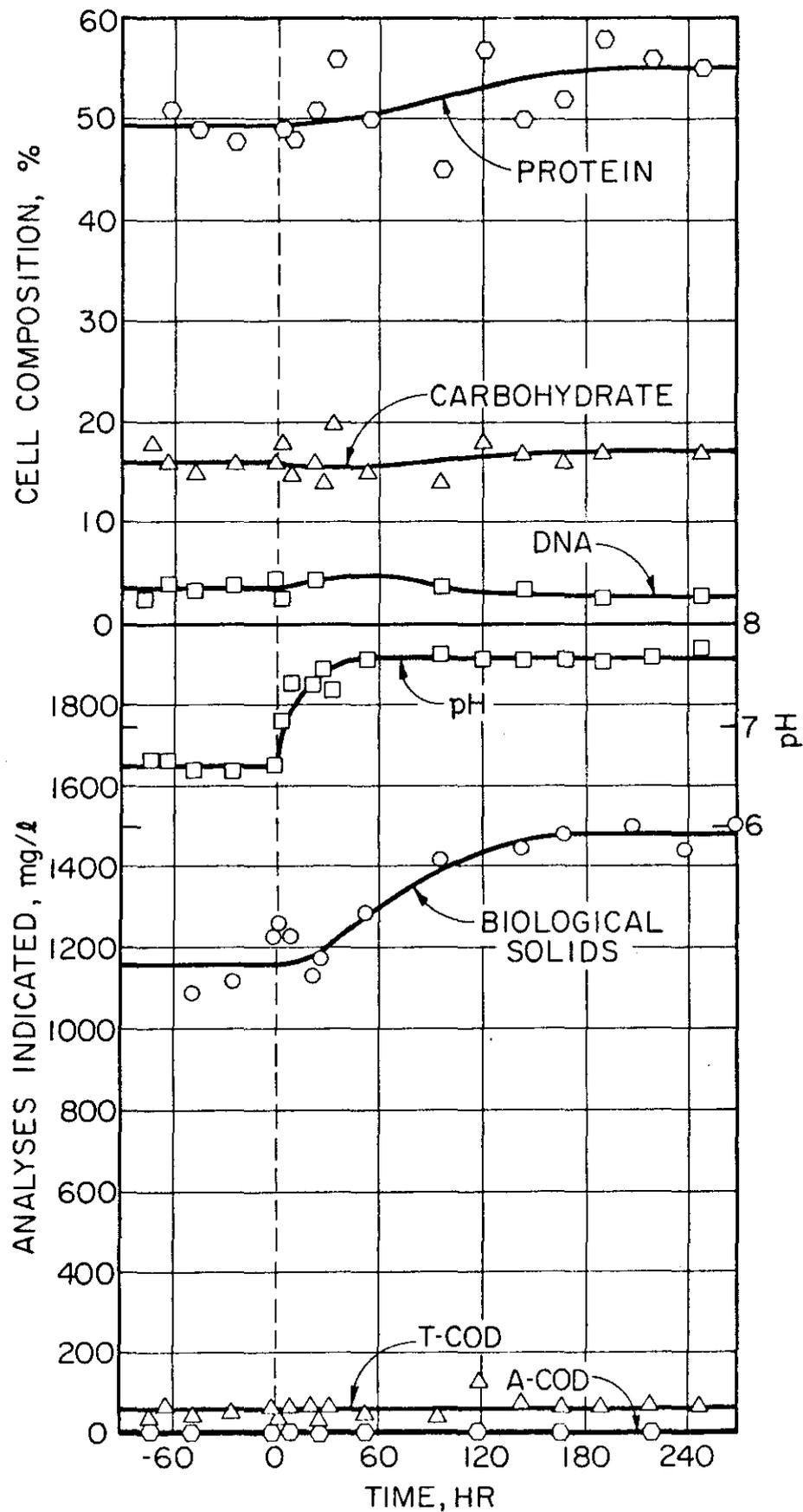
Figure 2. Response to an increase in pH from 6.6 to 7.7 ( $3500 \pm 350$  mg/l cells recycled at 33.3 percent of feed flow).
