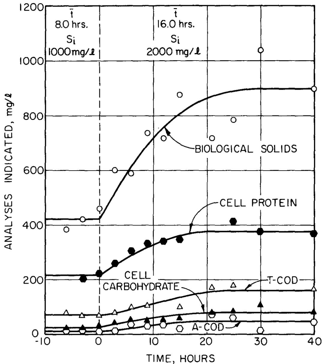
Figure 10. Response to decrease in dilution rate from  $0.125 \text{ hrs}^{-1}$ ,  $S_i = 1000 \text{ mg/l}$  glucose to  $0.062 \text{ hrs}^{-1}$ ,  $S_i = 2000 \text{ mg/l}$  glucose.
