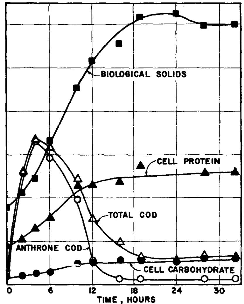
FIGURE 3. RESPONSE TO SHOCK LOAD;  $S_i$  1000→5000 mg/l AT  $\bar{t} = 4$  HOURS;
