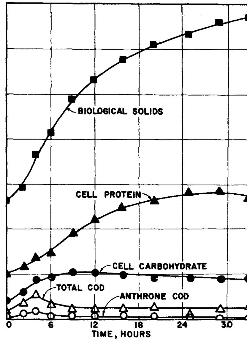
FIGURE 5. RESPONSE TO SHOCK LOAD;  $S_i$  1000  $\rightarrow$  3000 mg/l AT  $\bar{t} = 8$  HOURS;
