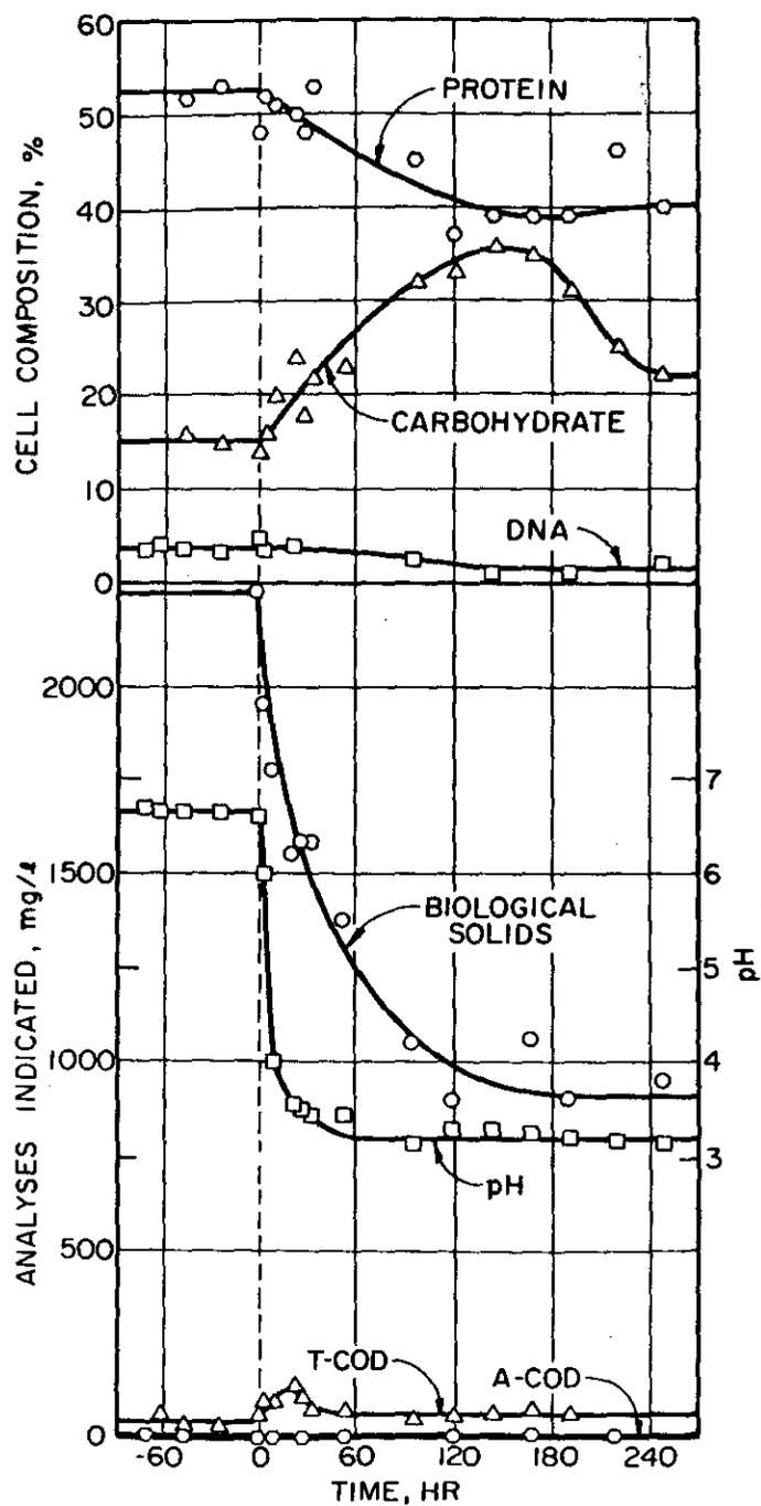
Figure 17. Response to a decrease in pH from 6.7 to 3.2 (total recycle of all settleable cells at 33% of feed flow).
