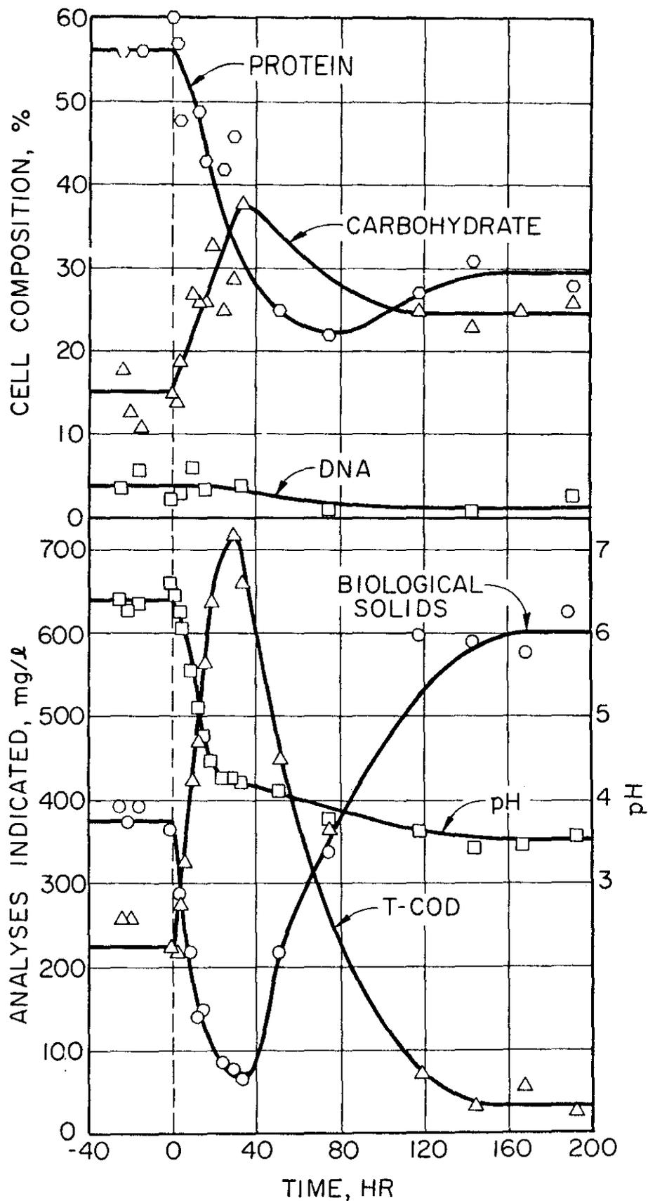
Figure 5. Response to a decrease in pH from 6.4 to 3.5 (no cell recycle).
