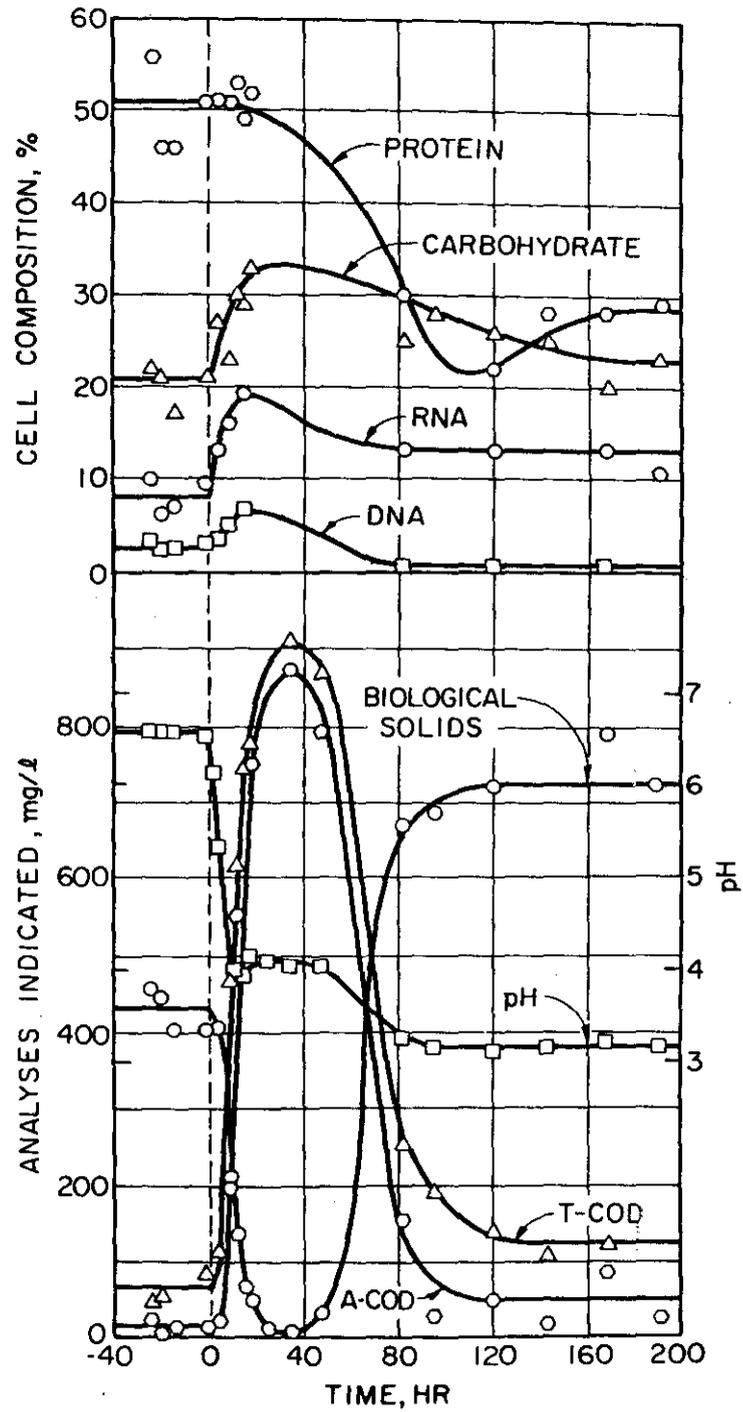
Figure 14. Response to a decrease in pH from 6.6 to 3.2 (no cell recycle).
