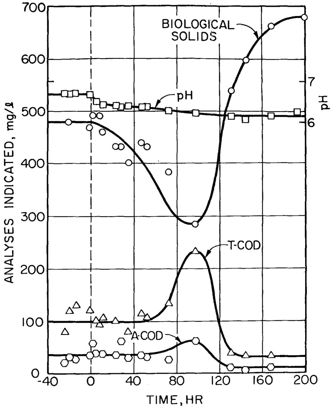
Figure 11. Response to a decrease in pH from 6.7 to 6.2 (no cell recycle).
