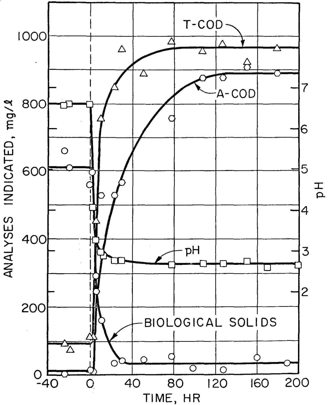
Figure 10. Response to a decrease in pH from 6.6 to 2.7 (no cell recycle).
