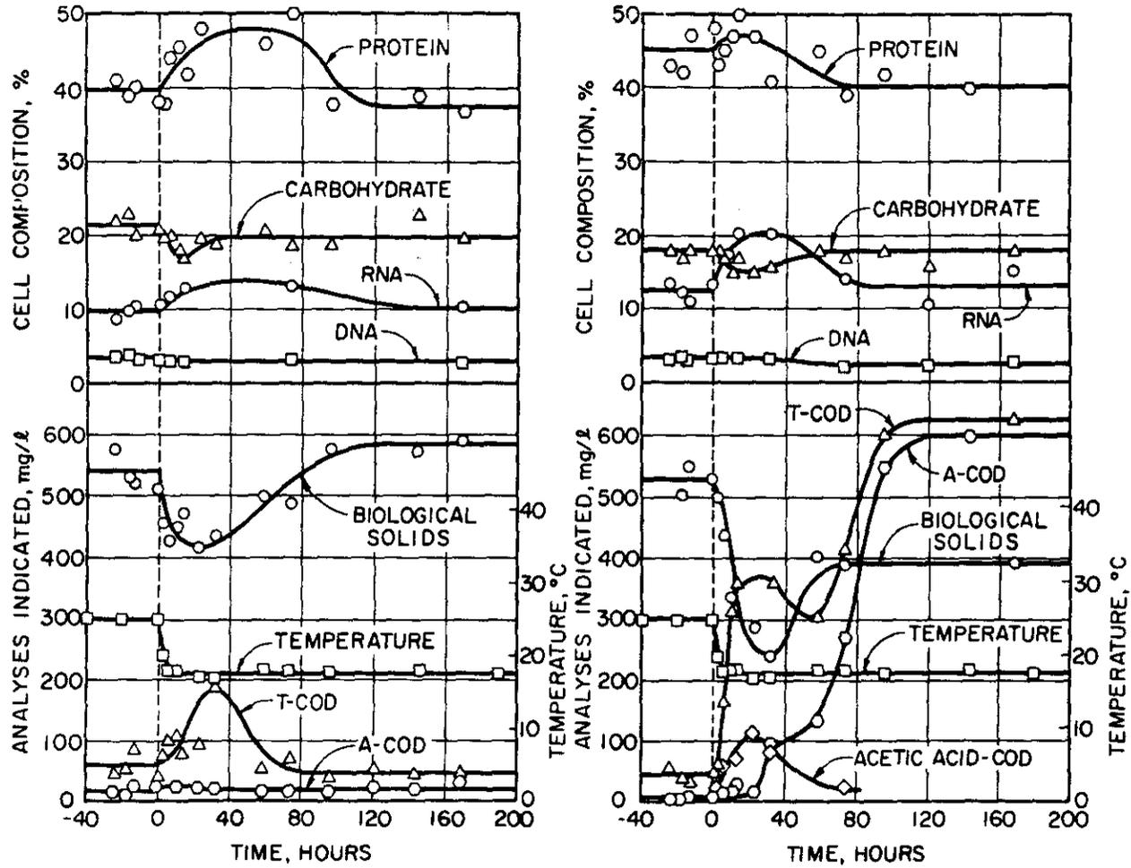
Figure 18. Response of a heterogeneous microbial population growing in a chemostat at 25° C to a decrease in temperature to 17.5° C. Left, dilution rate = 0.125 hrs<sup>-1</sup>; Right, dilution rate = 0.25 hrs<sup>-1</sup>.
