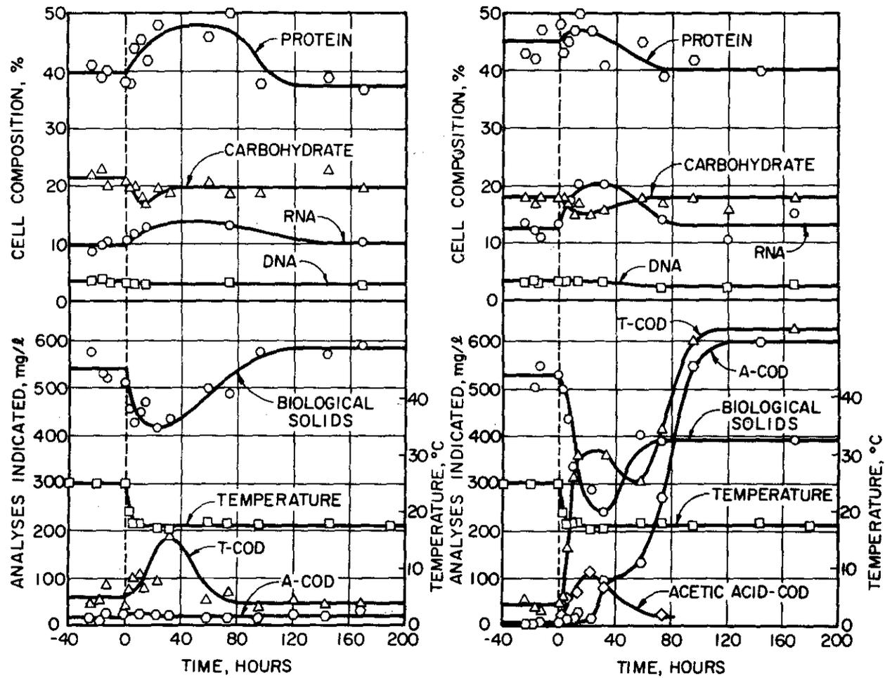
Figure 4. Response of a Heterogeneous Microbial Population Growing in a Once-through Chemostat at 25 C to a Decrease in Temperature to 17.5 C. Left, Dilution Rate = 0.125 hr<sup>-1</sup>; Right, Dilution Rate = 0.25 hr<sup>-1</sup>.
