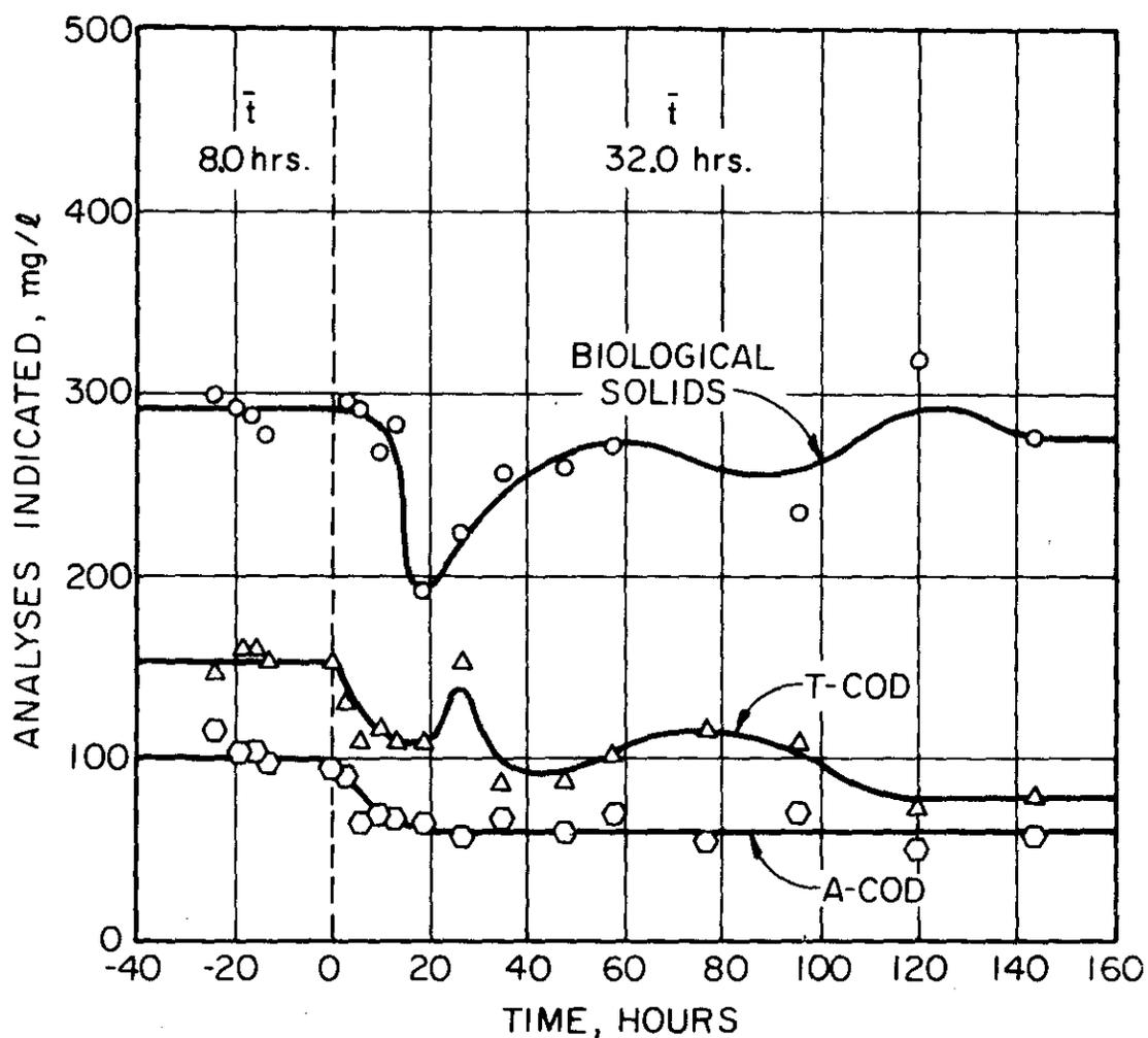
Figure 3. Response to decrease in dilution rate from  $0.125 \text{ hrs}^{-1}$  to  $0.031 \text{ hrs}^{-1}$ ;  $S_i = 1000 \text{ mg/l}$  glucose; T-COD is total chemical oxygen demand; A-COD is total carbohydrate (anthrone-reactive material) calculated as COD.
