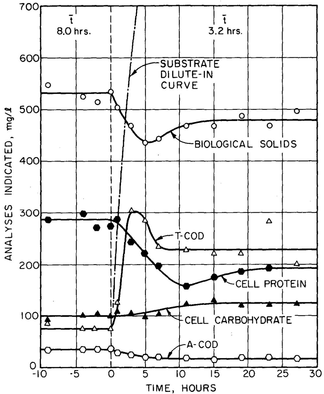
Figure 6. Response to increase in dilution rate from  $0.125 \text{ hrs}^{-1}$  to  $0.313 \text{ hrs}^{-1}$ ;  $S_j = 1000 \text{ mg/l}$  glucose.
