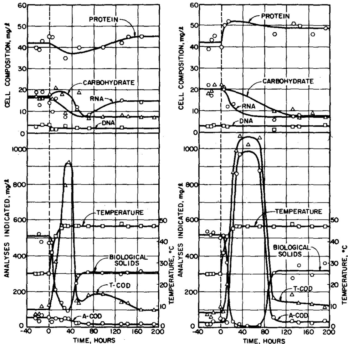
Figure 5. Response of a Heterogeneous Microbial Population Growing in a Once-through Chemostat at 25 C to an Increase in Temperature to 47 C. Left, Dilution Rate = 0.125 hr<sup>-1</sup>; Right, Dilution Rate = 0.25 hr<sup>-1</sup>.
