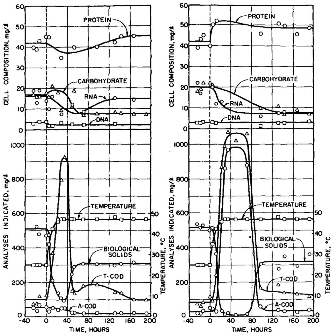
Figure 20. Response of a heterogeneous microbial population growing in a chemostat at 25° C to an increase in temperature to 47° C. Left, dilution rate = 0.125 hrs<sup>-1</sup>; Right, dilution rate = 0.25 hrs<sup>-1</sup>.
