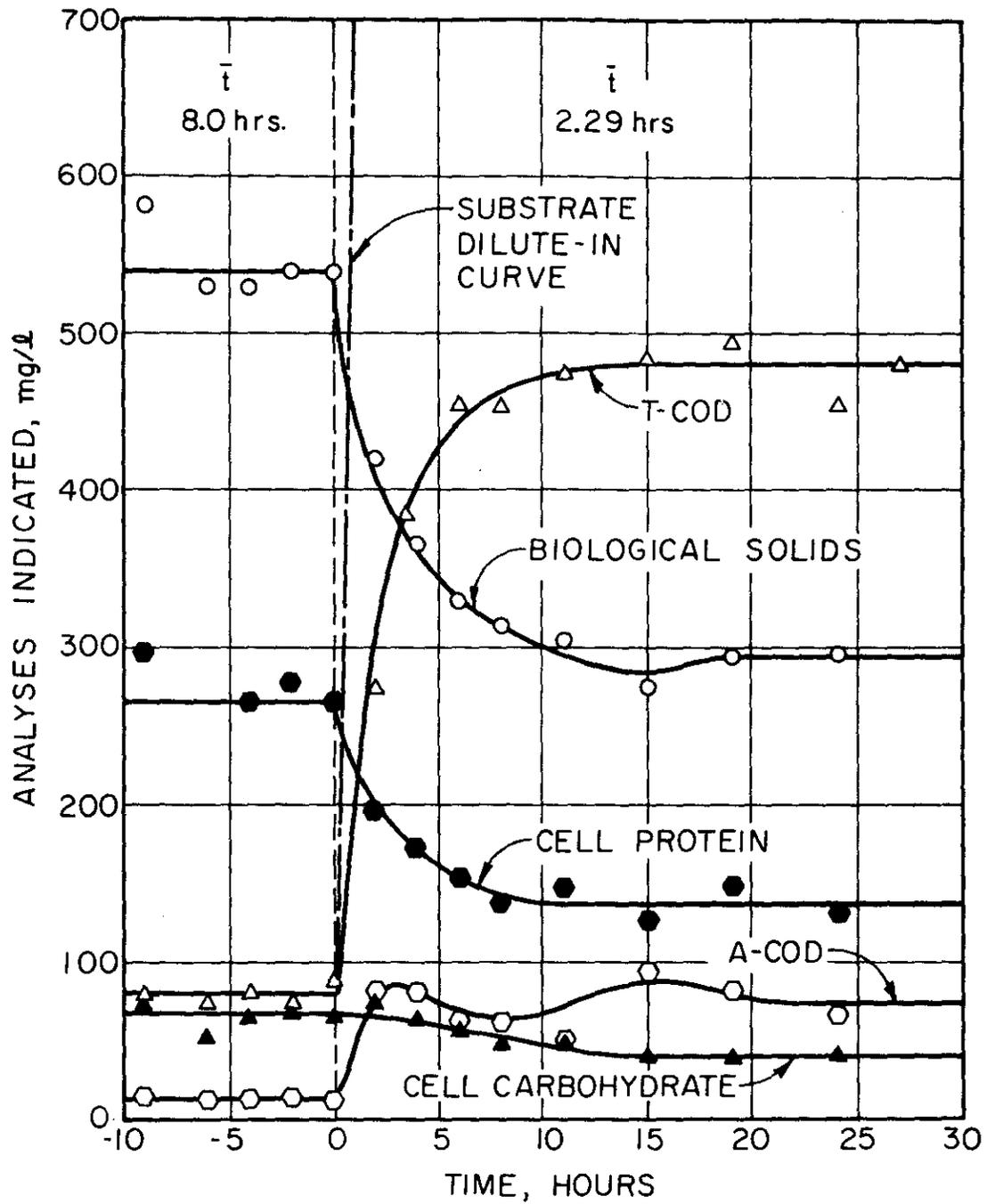
Figure 8. Response to increase in dilution rate from  $0.125 \text{ hrs}^{-1}$  to  $0.437 \text{ hrs}^{-1}$ ;  $S_i = 1000 \text{ mg/l}$  glucose.
