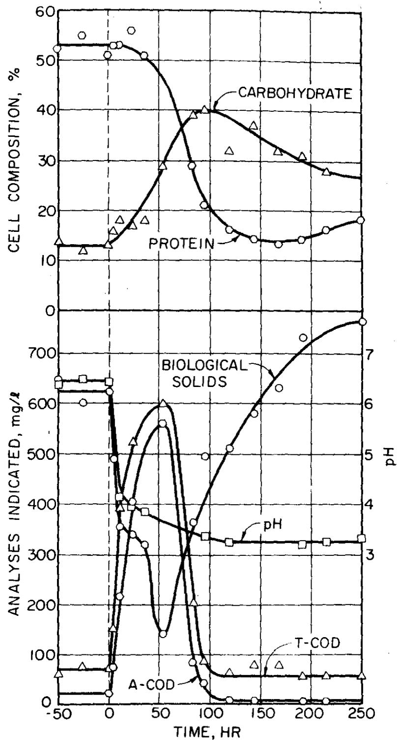
Figure 2. Response of a Heterogeneous Microbial Population Growing in a Chemostat to a Decrease in pH from 6.5 to 3.3 ( $\pm 1000$  mg/l Cells Recycled at 33.3 Percent of Feed Flow)
