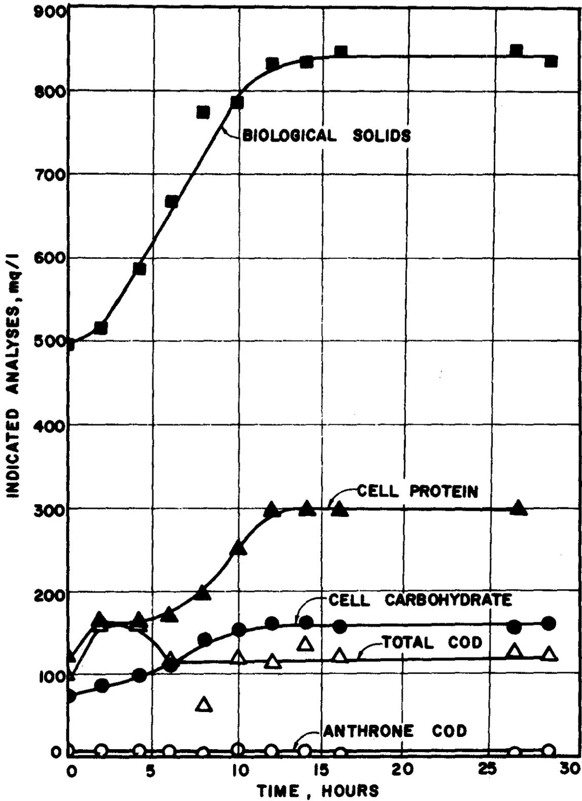
FIGURE 4. RESPONSE TO SHOCK LOAD;  $S_i$  1000-2000 mg/l AT  $\bar{t} = 8$  HOURS; ONCE THROUGH SYSTEM
