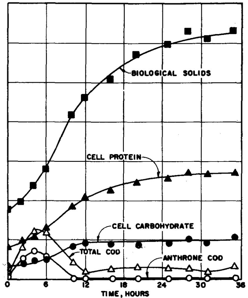
FIGURE 9. RESPONSE TO SHOCK LOAD;  $S_i$  1000  $\rightarrow$  5000 mg/l AT  $\bar{t} = 12$  HOURS; LEFT: ONCE THROUGH, RIGHT: CELL RECYCLE
