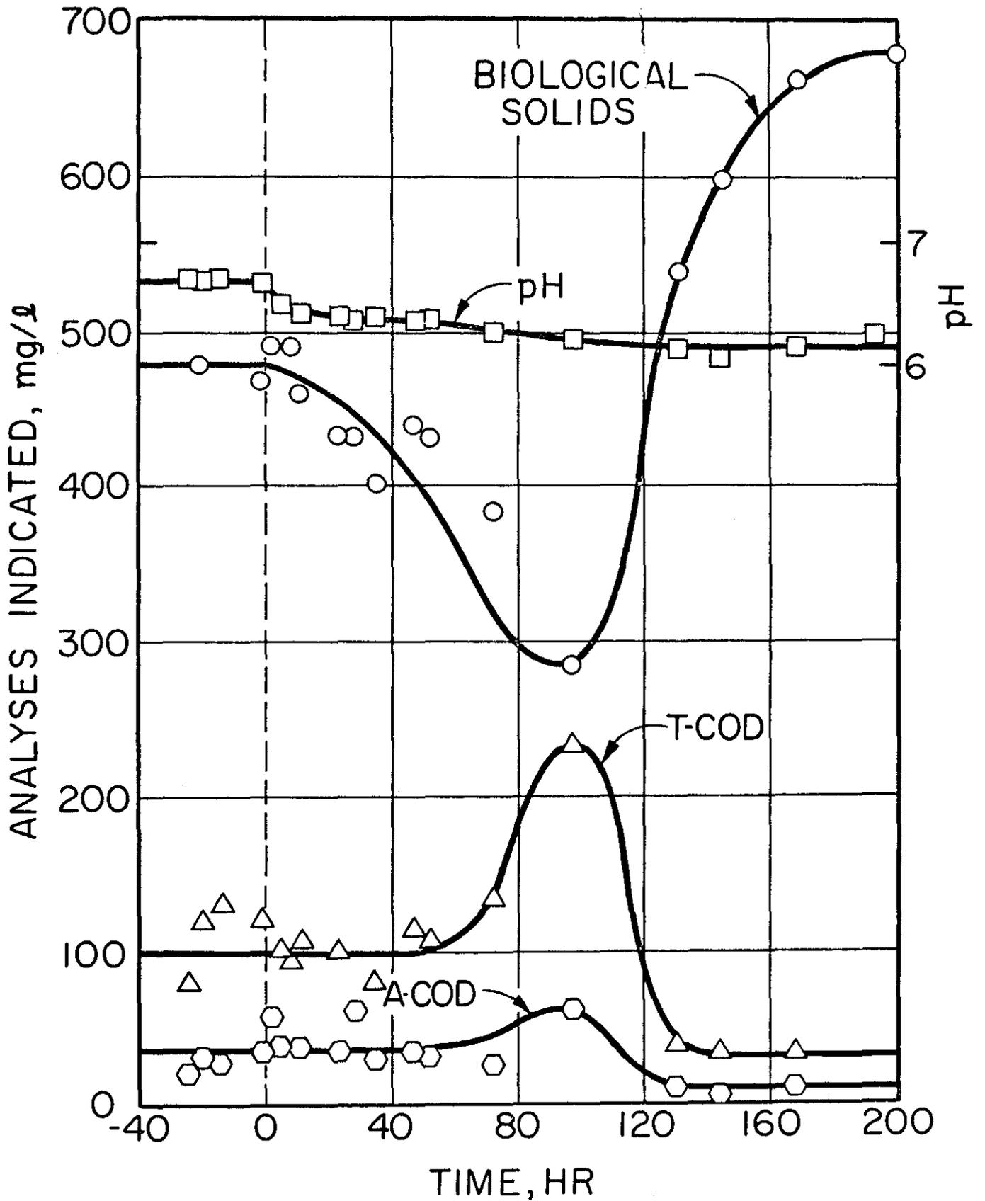
Figure 3. Response to a decrease in pH from 6.7 to 6.2 (no cell recycle).
