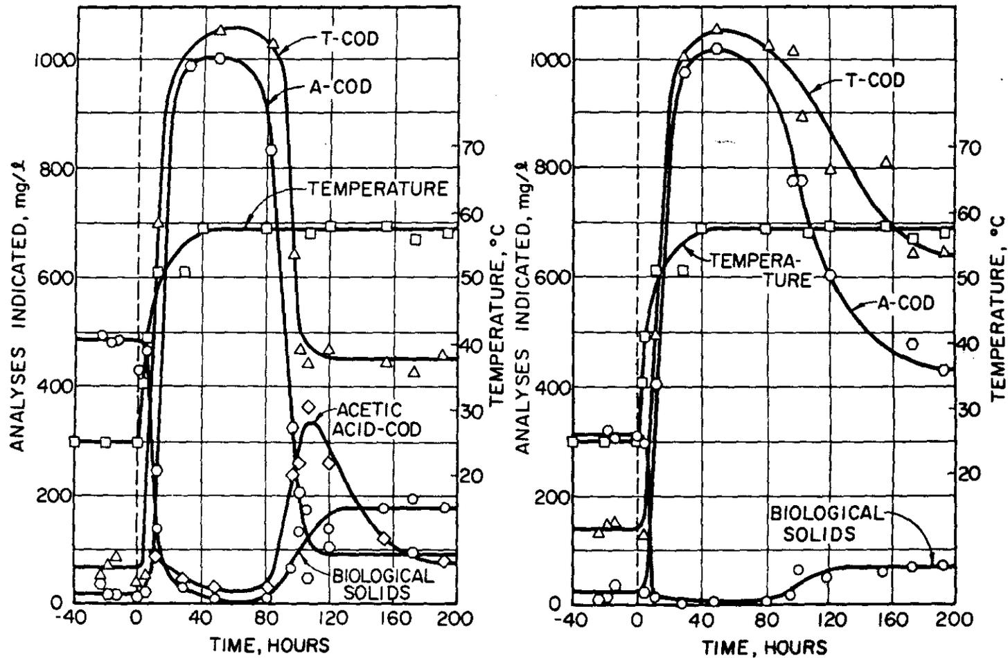
Figure 21. Response of a heterogeneous microbial population growing in a chemostat at 25° C to an increase in temperature to 57.5° C. Left, dilution rate = 0.125 hrs<sup>-1</sup>; Right, dilution rate = 0.25 hrs<sup>-1</sup>.
