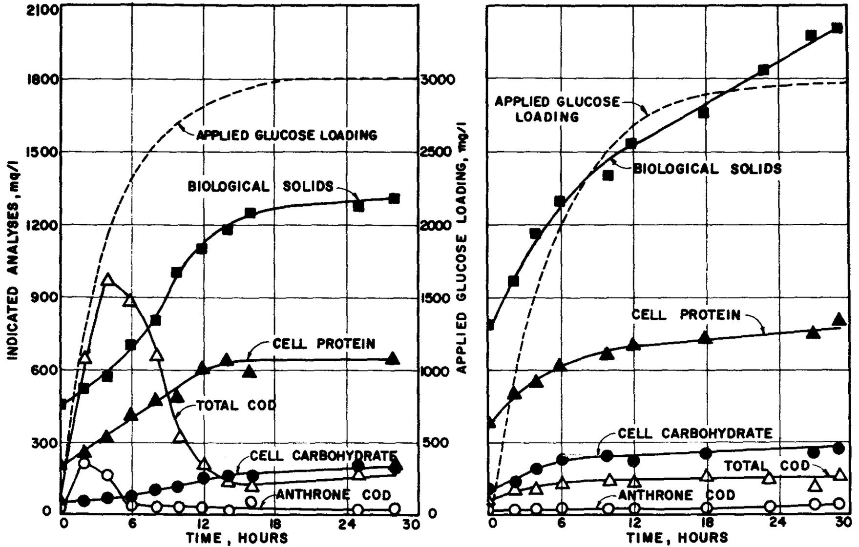
FIGURE 2. RESPONSE TO SHOCK LOAD;  $S_i$  1000-3000 mg/l AT  $\bar{t} = 4$  HOURS;
