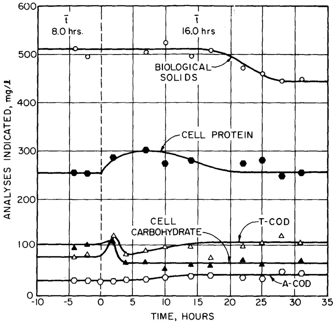
Figure 4. Response to decrease in dilution rate from  $0.125 \text{ hrs}^{-1}$  to  $0.062 \text{ hrs}^{-1}$ ;  $S_i = 1000 \text{ mg/l}$  glucose.
