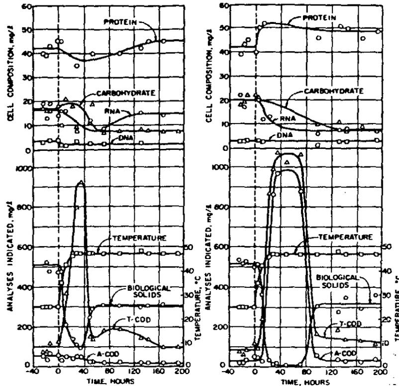
FIG. 4. Response of a heterogeneous microbial population growing in a chemostat at 25 C to an increase in temperature to 47 C. Left, dilution rate = 0.125 per h; right, dilution rate = 0.25 per h.
