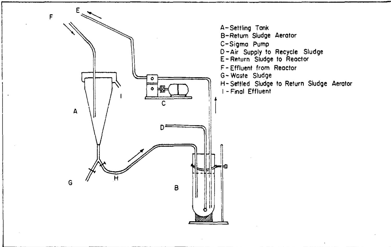
Figure 2. Side view of sludge recycle system added to pilot plant shown in Figure 1 for studies employing cell feedback to reactor.
