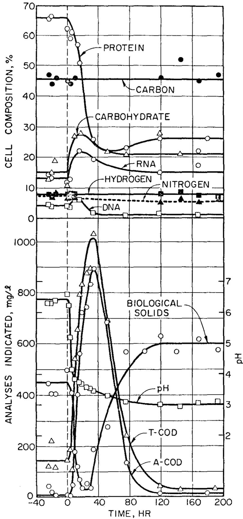
Figure 9. Response to a decrease in pH from 6.5 to 3.0 (no cell recycle).
