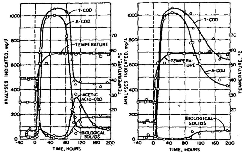
FIG. 5. Response of a heterogeneous microbial population growing in a chemostat at 25 C to an increase in temperature at 57.5 C. Left, dilution rate = 0.125 per h; right, dilution rate = 0.25 per h.
