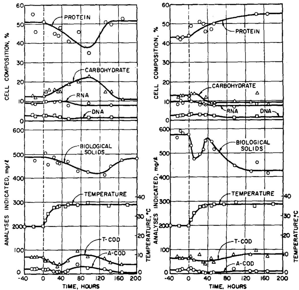
Figure 19. Response of a heterogeneous microbial population growing in a chemostat at  $25^{\circ}\text{C}$  to an increase in temperature to  $36^{\circ}\text{C}$ . Left, dilution rate =  $0.125\text{ hrs}^{-1}$ ; Right, dilution rate =  $0.25\text{ hrs}^{-1}$ .
