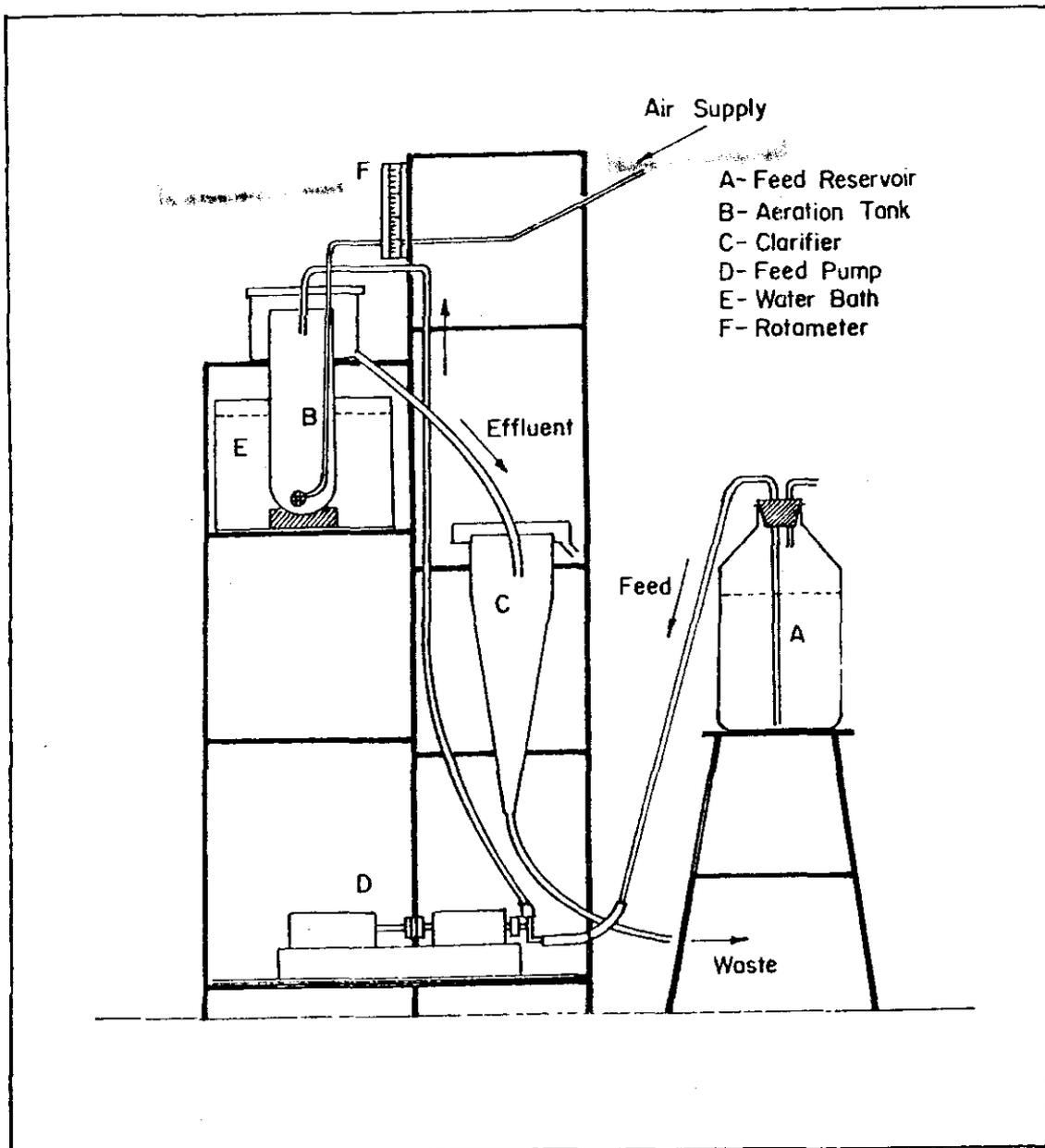
Figure 1. Side view of completely mixed continuous flow reactor employed in laboratory studies of "once-through" systems. A, feed reservoir; B, aeration tank; C, clarifier, D, feed pump; E, water bath; F, rotameter.
