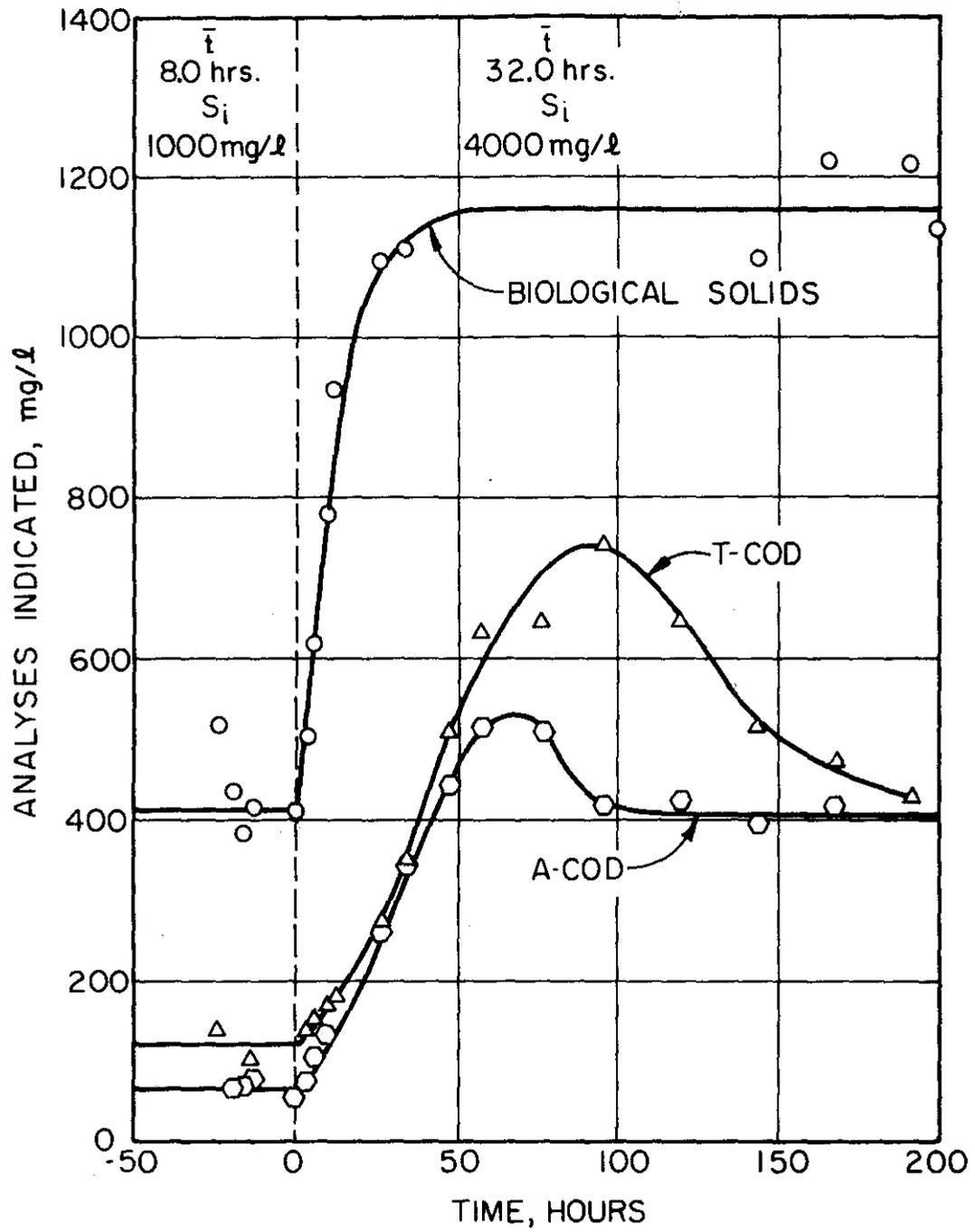
Figure 9. Response to decrease in dilution rate from  $0.125 \text{ hrs}^{-1}$ ,  $S_i = 1000 \text{ mg/l}$  glucose to  $0.031 \text{ hrs}^{-1}$ ,  $S_i = 4000 \text{ mg/l}$  glucose.
