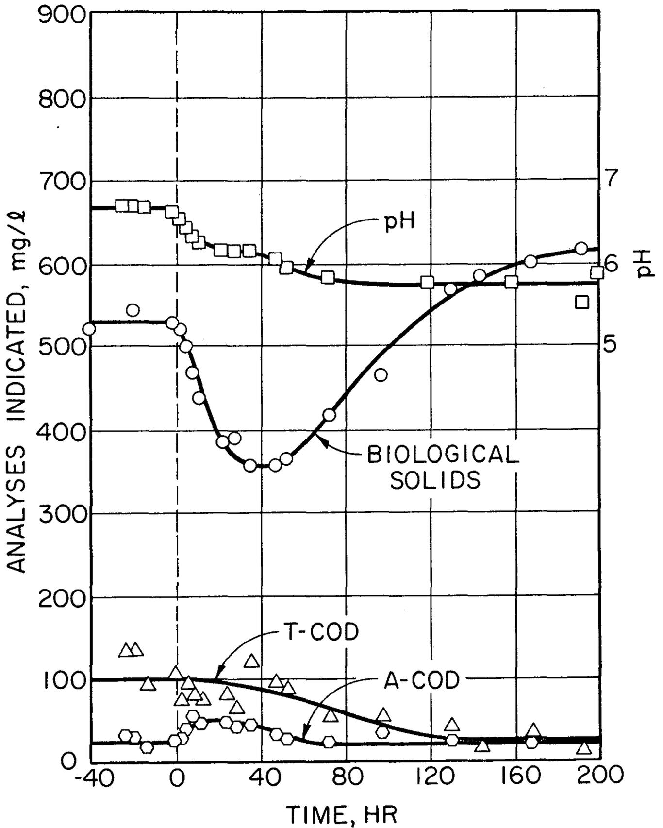
Figure 4. Response to a decrease in pH from 6.7 to 5.8 (no cell recycle).
