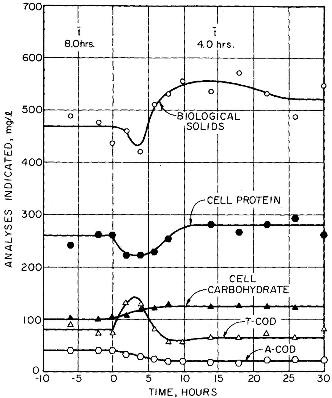
Figure 5. Response to increase in dilution rate from  $0.125 \text{ hrs}^{-1}$  to  $0.25 \text{ hrs}^{-1}$ ;  $S_i = 1000 \text{ mg/l}$  glucose.
