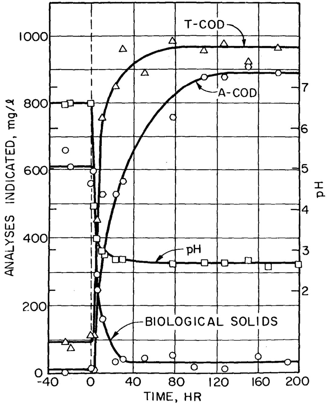
Figure 16. Response to a decrease in pH from 6.6 to 2.7 (no cell recycle).
