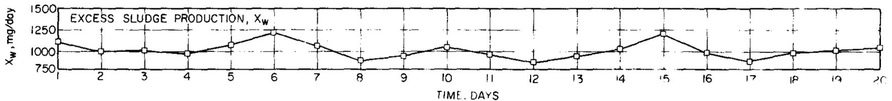
Figure 3 OPERATIONAL CHARACTERISTICS FOR AN ACTIVATED SLUDGE PROCESS WITH CONSTANT  $X_R$  AT AN  $S_i$  OF 500 mg/l
