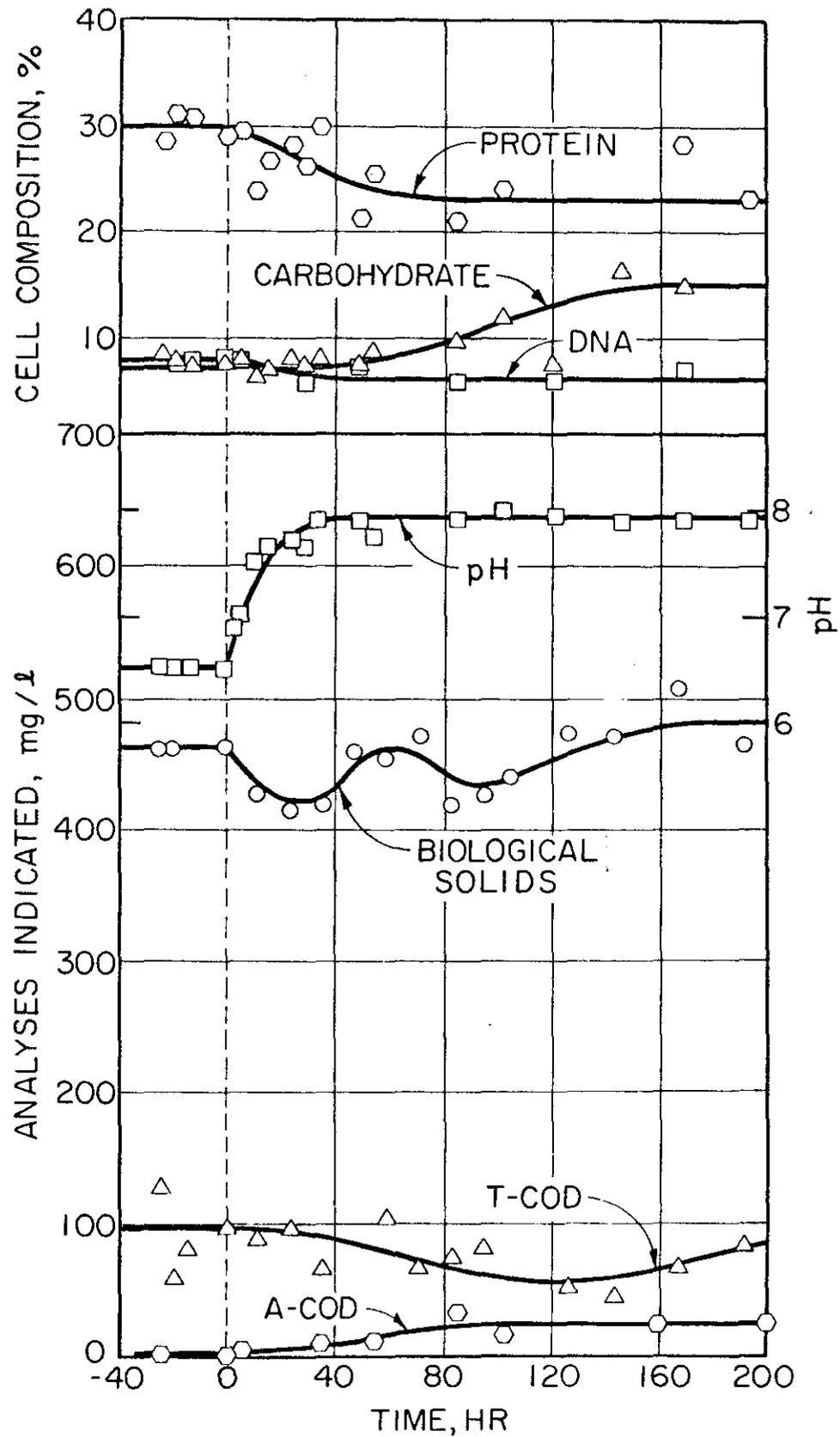
Figure 1. Response to an increase in pH from 6.6 to 8.0 (no cell recycle). T-COD is total COD of filtered effluent, and A-COD is total anthrone-reactive material (carbohydrate) in filtered effluent calculated as COD.
