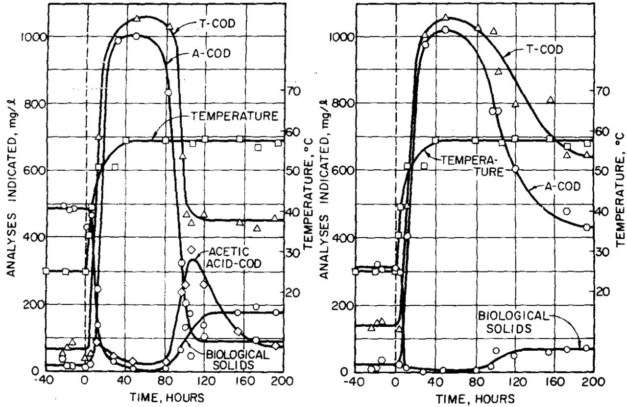
Figure 6. Response of a Heterogeneous Microbial Population Growing in a Once-through Chemostat at 25 C to an Increase in Temperature to 57.5 C. Left, Dilution Rate =  $0.125 \text{ hr}^{-1}$ ; Right, Dilution Rate =  $0.25 \text{ hr}^{-1}$ .
