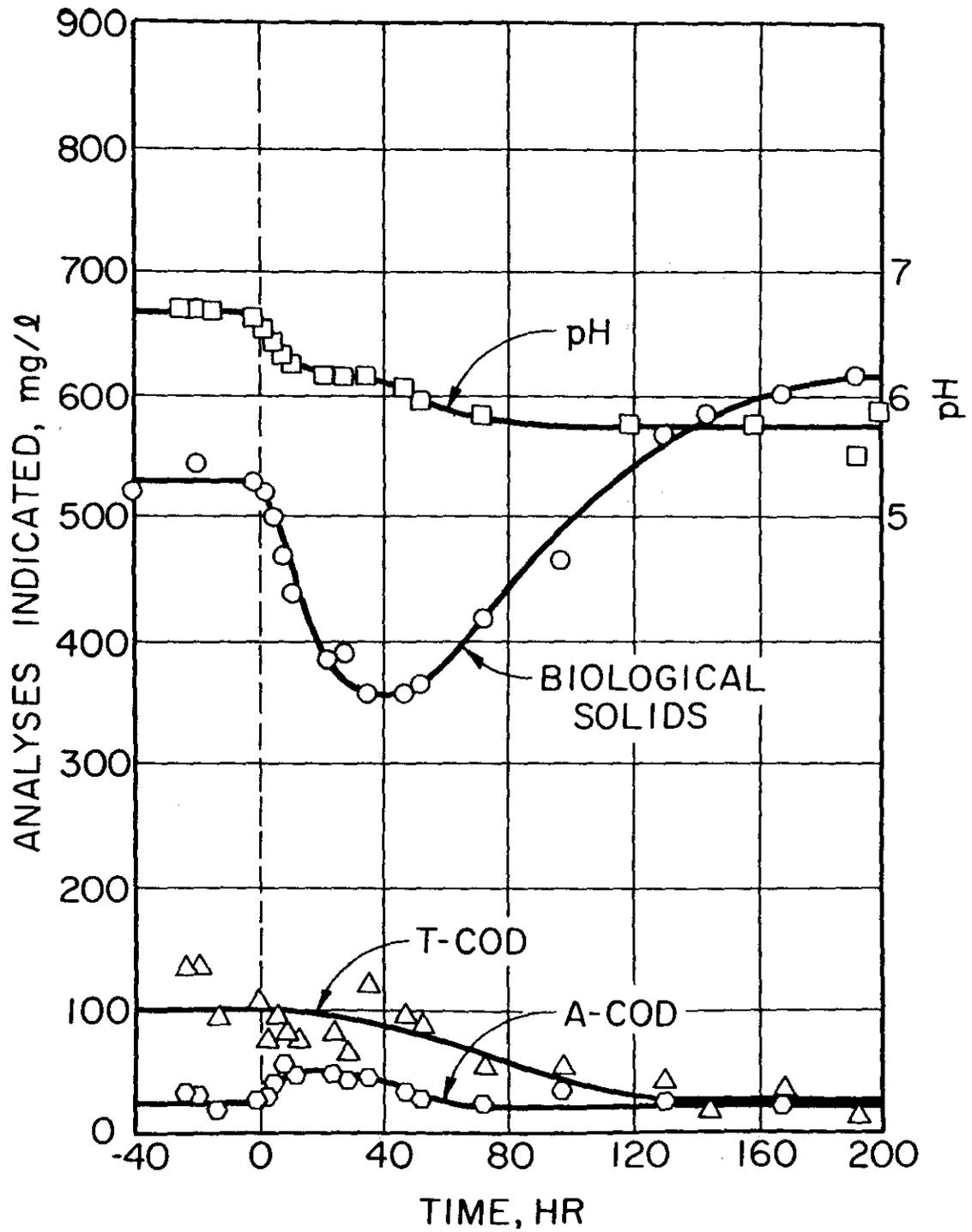
Figure 12. Response to a decrease in pH from 6.7 to 5.8 (no cell recycle).
