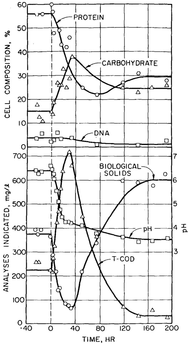
Figure 13. Response to a decrease in pH from 6.4 to 3.5 (no cell recycle).
