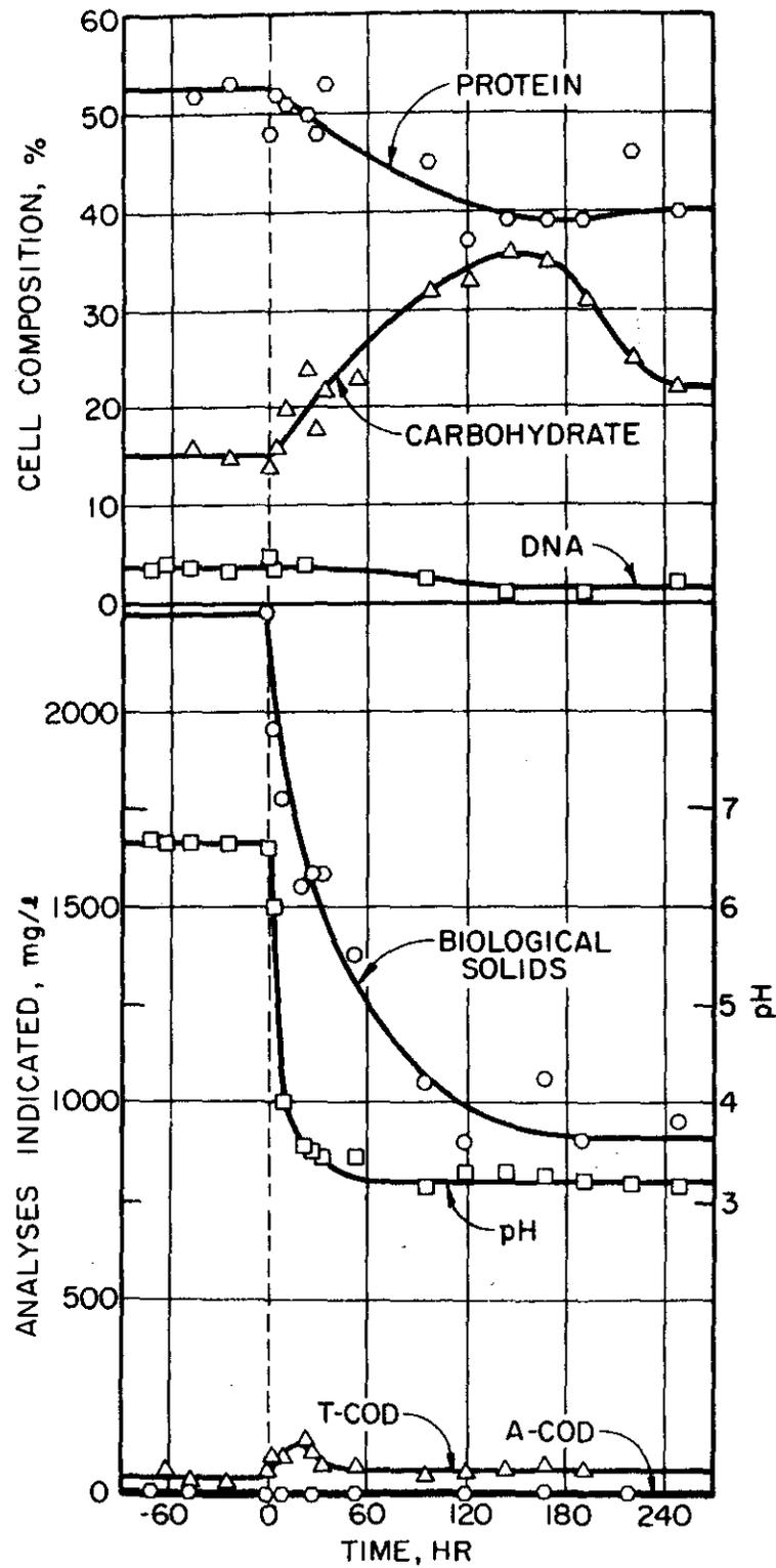
Figure 3. Response of a Heterogeneous Microbial Population Growing in a Chemostat to a Decrease in pH from 6.7 to 3.2 (total recycle of all settleable cells at 33.3 percent of feed flow)
