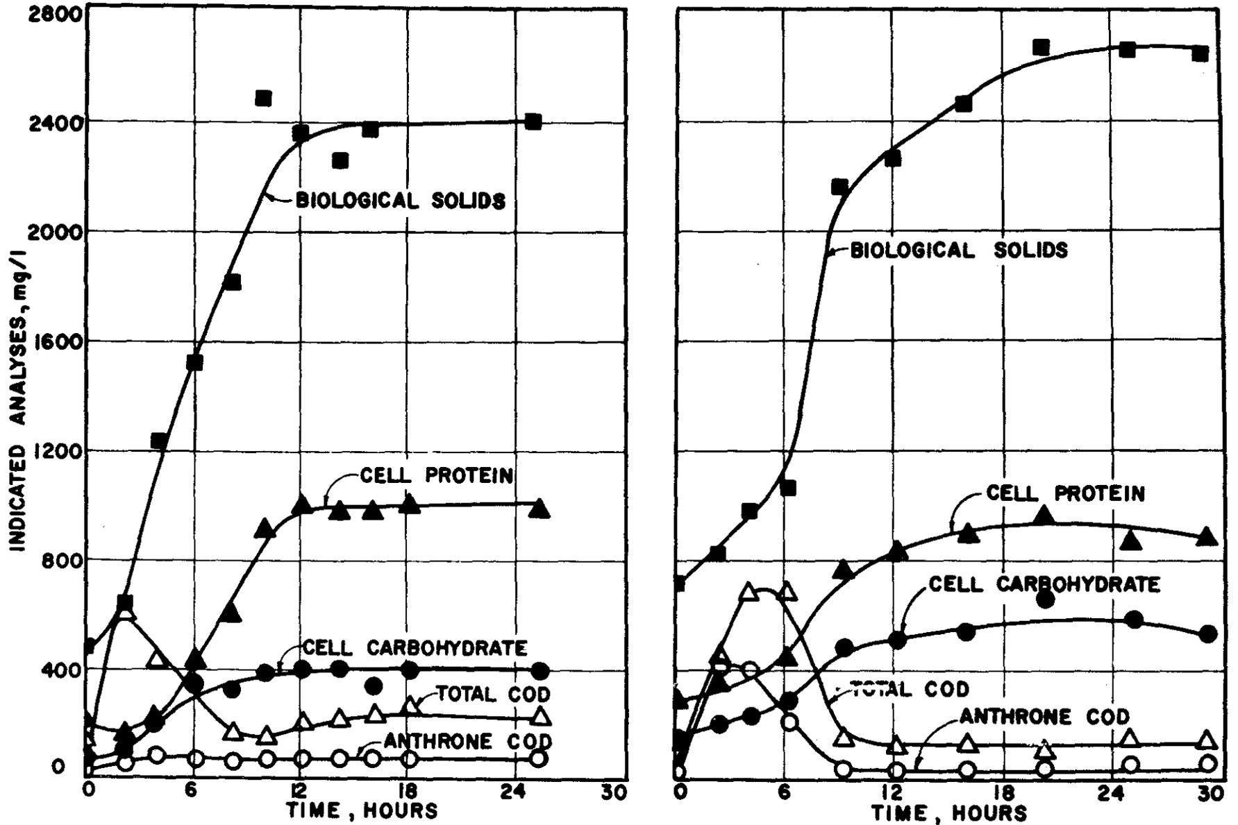
FIGURE 6. RESPONSE TO SHOCK LOAD;  $S_i$  1000  $\rightarrow$  5000 mg/l AT  $\bar{t} = 8$  HOURS; LEFT: ONCE THROUGH, RIGHT: CELL RECYCLE
