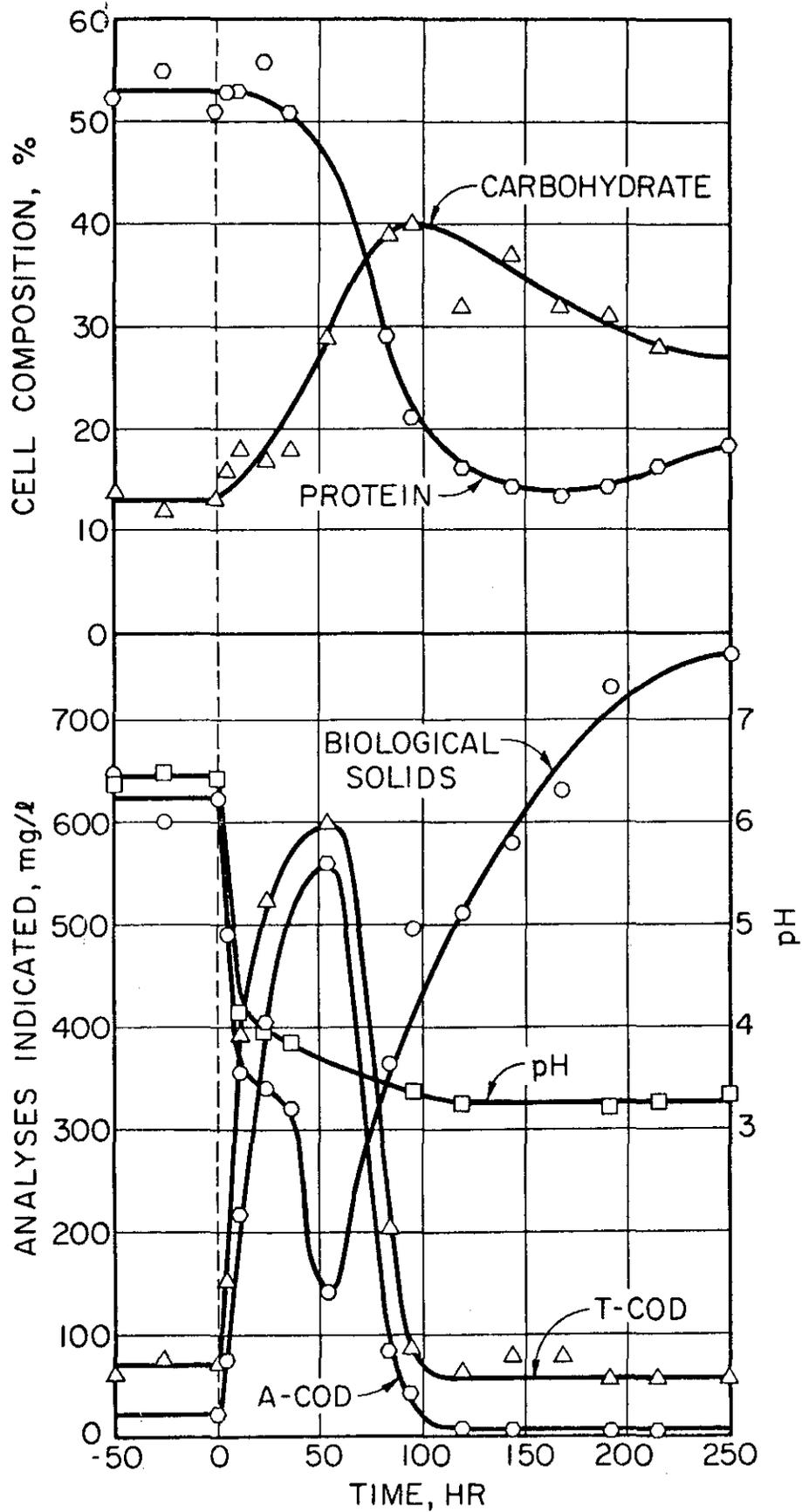
Figure 6. Response to a decrease in pH from 6.5 to 3.3 ( $\pm 1000$  mg/l cells recycled at 33.3 percent of feed flow).
