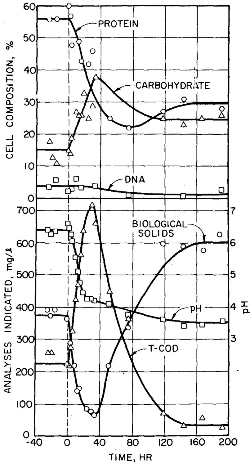
Figure 1. Response of a Heterogeneous Microbial Population Growing in a Once-through Chemostat to a Decrease in pH from 6.4 to 3.5
