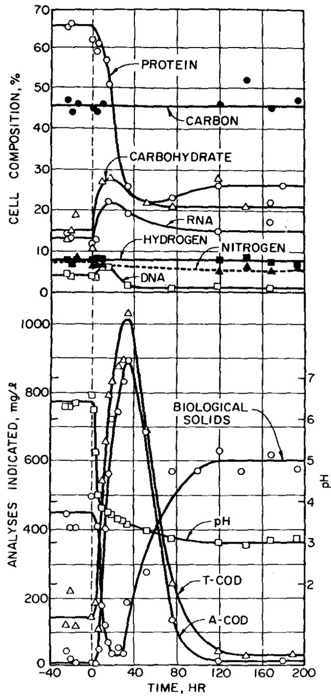
Figure 15. Response to a decrease in pH from 6.4 to 3.0 (no cell recycle).
