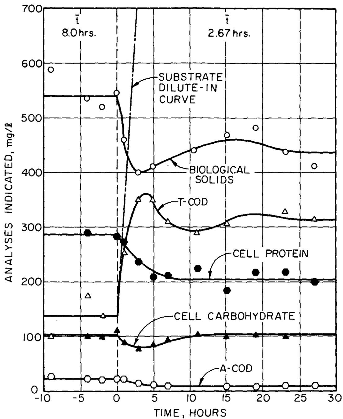
Figure 7. Response to increase in dilution rate from  $0.125 \text{ hrs}^{-1}$  to  $0.375 \text{ hrs}^{-1}$ ;  $S_i = 1000 \text{ mg/l}$  glucose.
