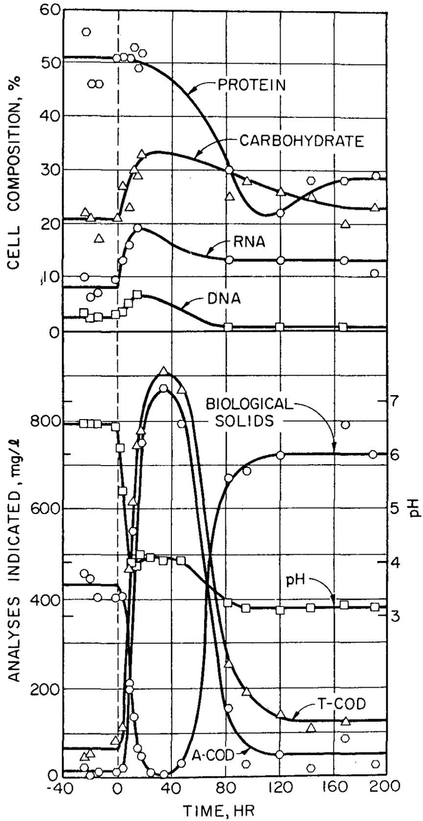
Figure 8. Response to a decrease in pH from 6.6 to 3.2 (no cell recycle).
