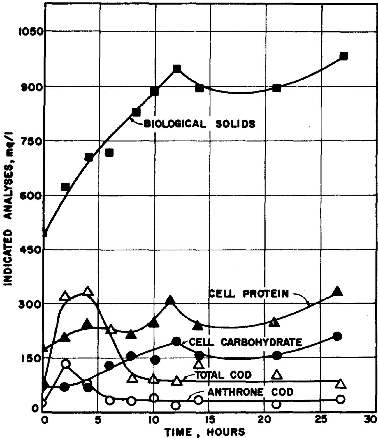
FIGURE 1. RESPONSE TO SHOCK LOAD;  $S_i$  1000 → 2000 mg/l AT  $\bar{t} = 4$  HOURS; ONCE THROUGH SYSTEM.
