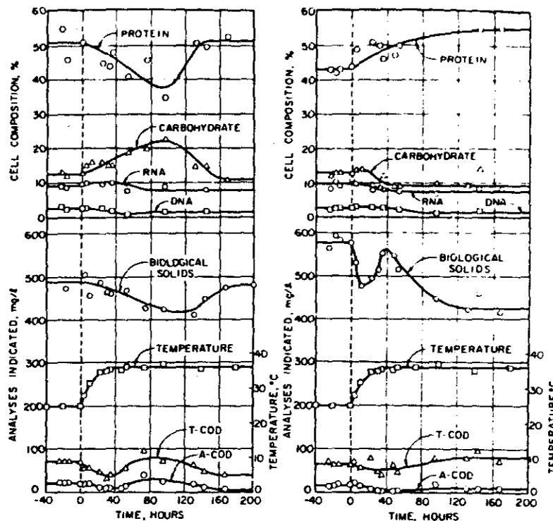
FIG. 3. Response of a heterogeneous microbial population growing in a chemostat at 25°C to an increase in temperature to 36°C. Left, dilution rate = 0.125 per h; right, dilution rate = 0.25 per h.
