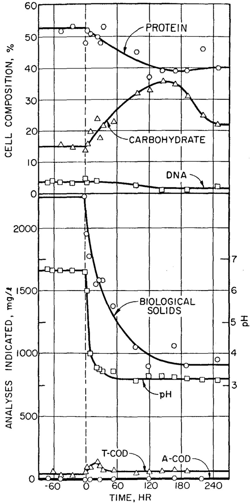
Figure 7. Response to a decrease in pH from 6.7 to 3.2 (total recycle of all settleable cells at 33.3 percent of feed flow).
