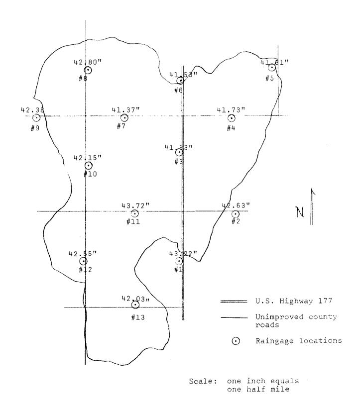
No. 7 recorded the smallest total precipitation which was 3.2% less than the mean. These two rain gages were near the center of the network and only 1 mile apart. No pattern of areal rainfall distribution was discernable.
