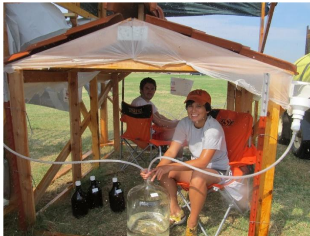
Figure 51. Collecting the composite sample during a rainfall simulation.
