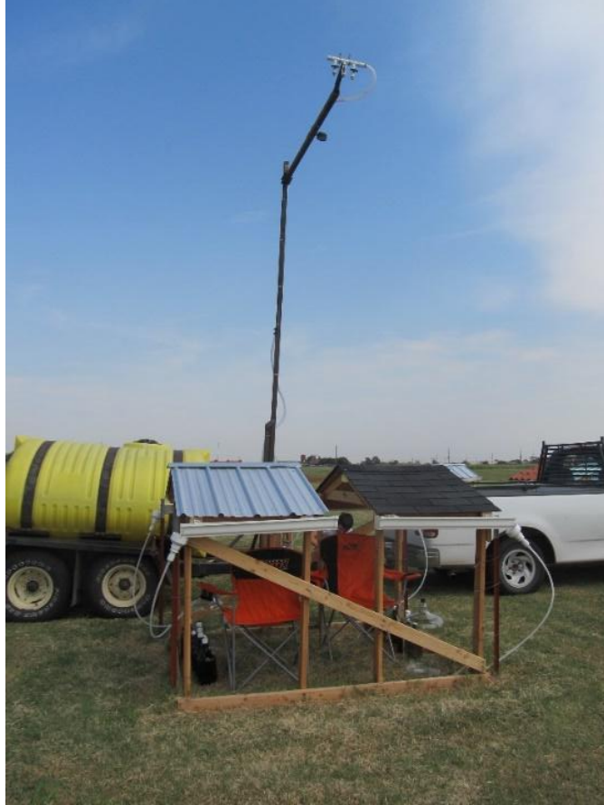
Figure 48. Rainfall simulator trailer with two constructed roofs.
