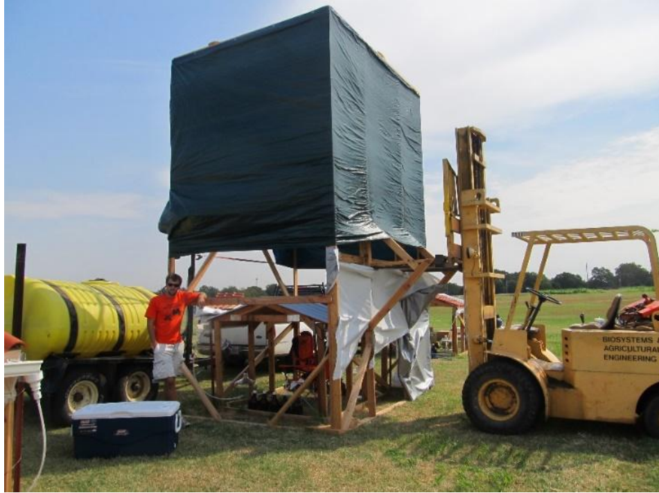
Figure 49. Wind block placement over constructed roofs before a simulation.
