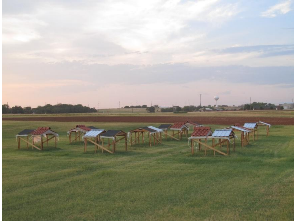
Figure 46. Constructed roof layout for rainfall simulations.
