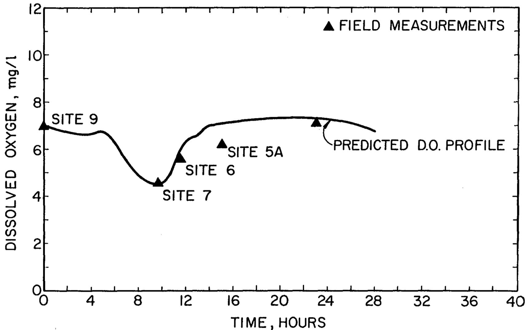
Figure 22. OXYGEN SAG CURVE FOR  $Q = 6$  cfs AND TIME OF TRAVEL BASED UPON MANNINGS EQUATION.
