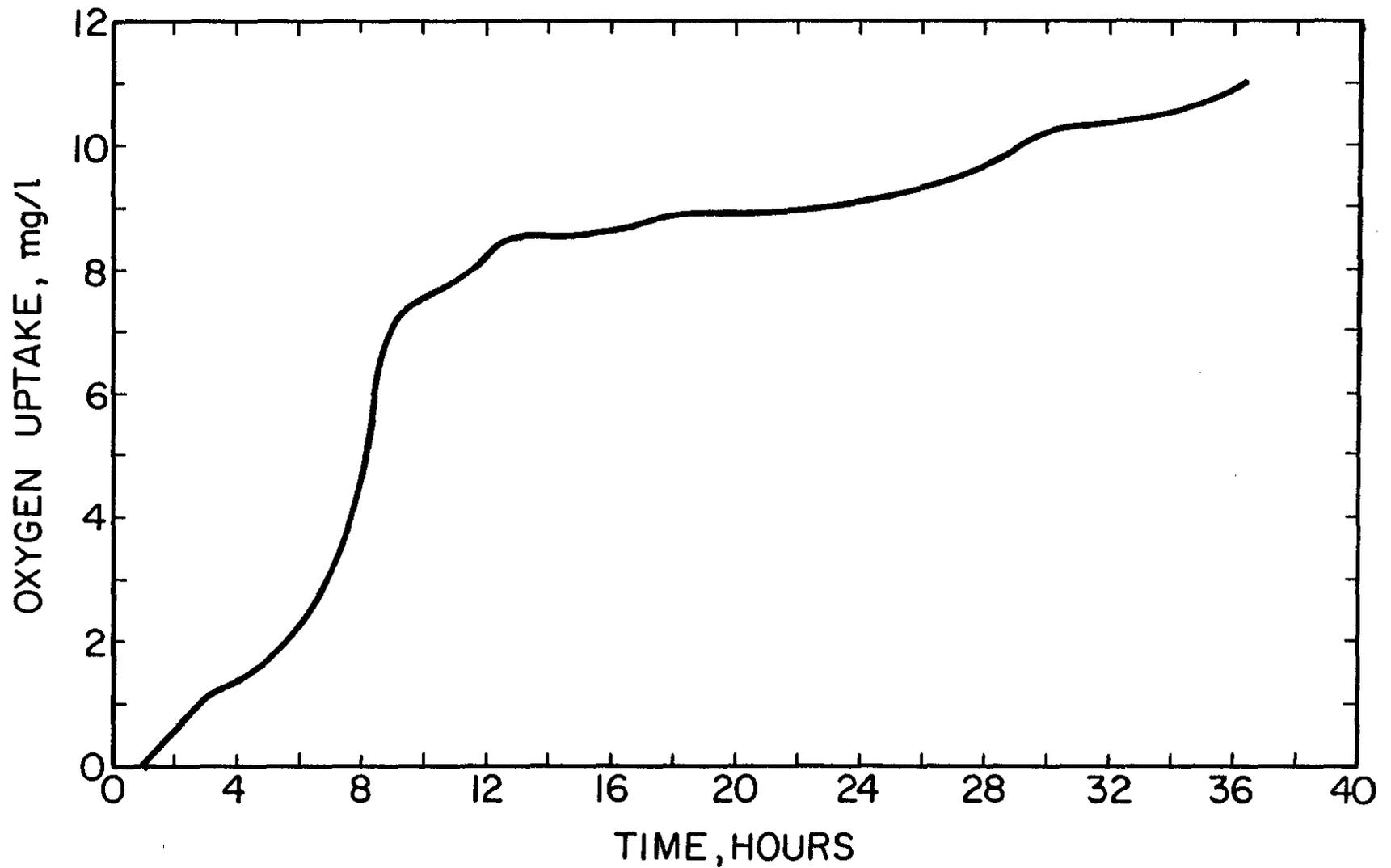
Figure 20. OXYGEN UPTAKE CURVE FOR  $k_2 = 0.069$  hr AND  $S_i = 50$  mg/l.
