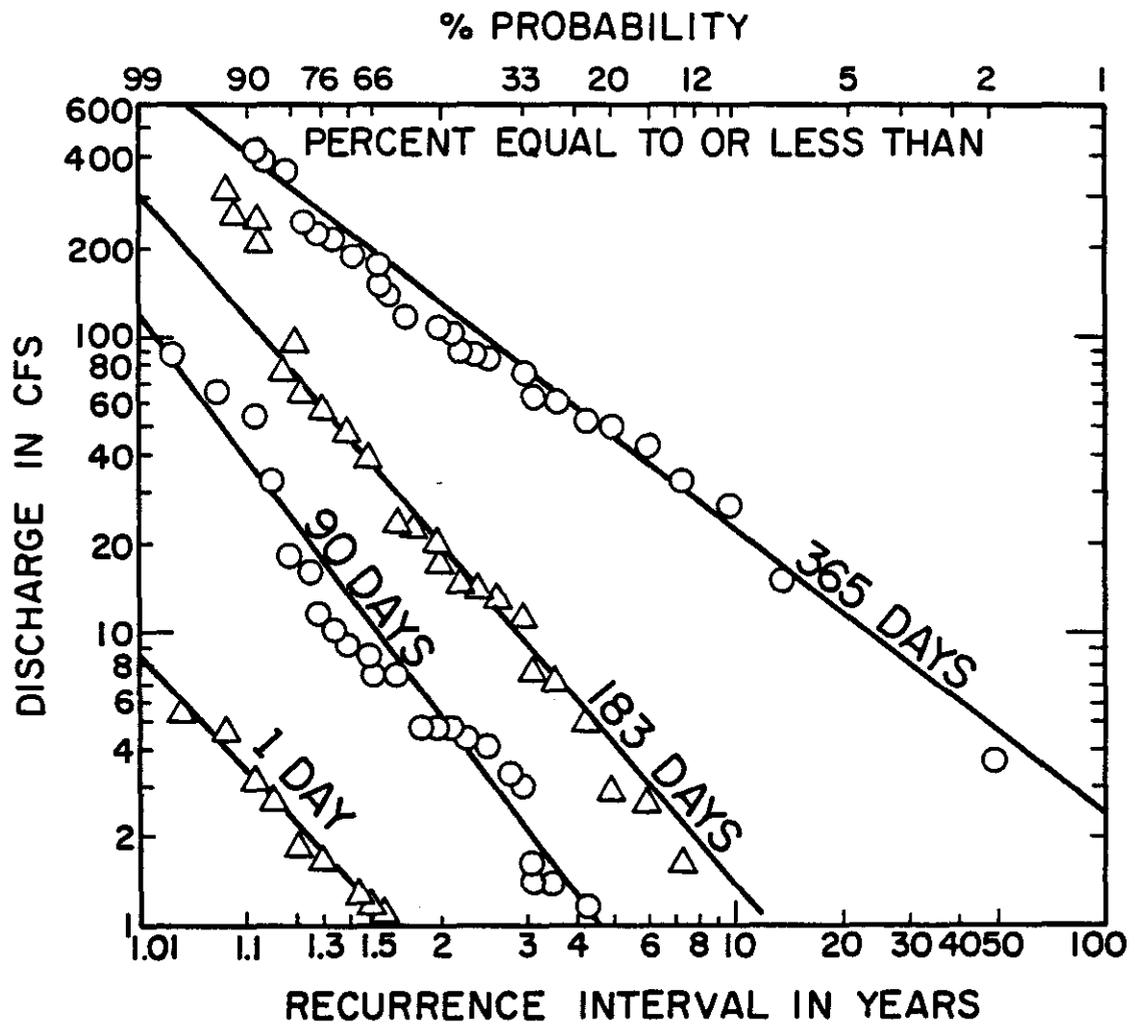
Figure 30. LOW FLOW FREQUENCY CURVE,
