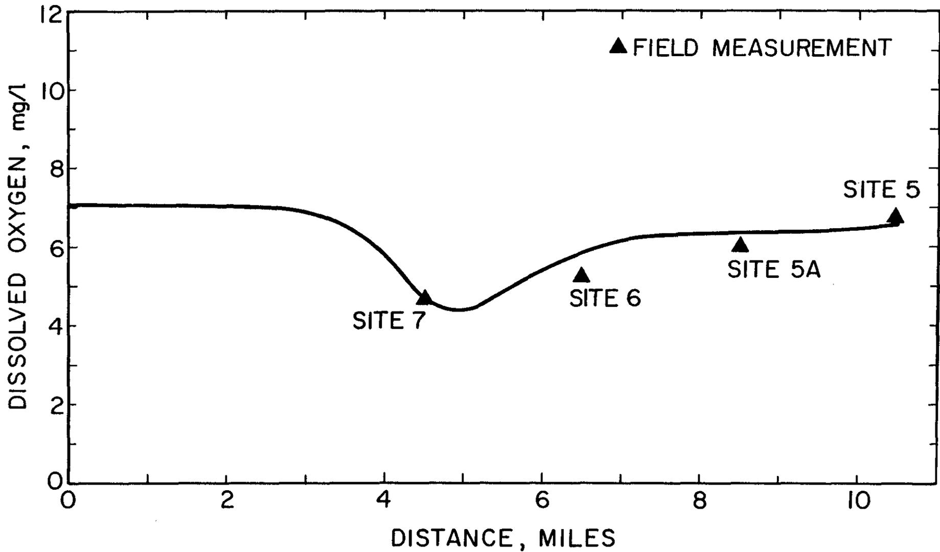
Figure 29. OXYGEN SAG CURVE VS. DISTANCE FOR Q = 2.6 cfs AND TIME OF TRAVEL BASED UPON OXYGEN SAG.
