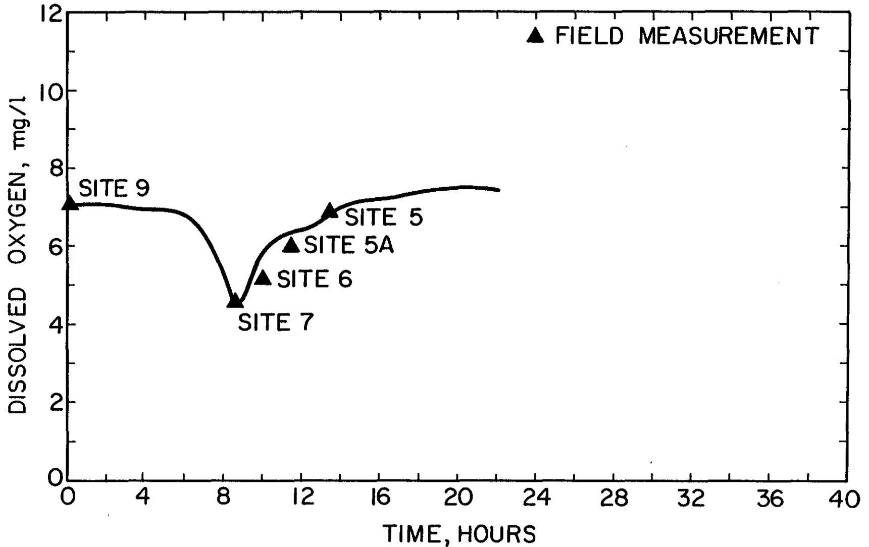
Figure 28. OXYGEN SAG CURVE FOR Q = 2.6 cfs AND TIME OF TRAVEL BASED UPON OXYGEN SAG.
