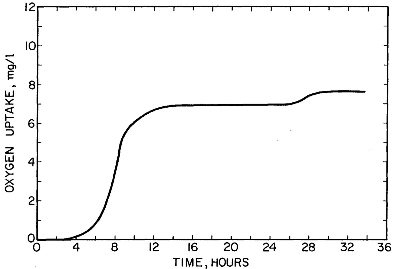
Figure 19. OXYGEN UPTAKE CURVE FOR  $K_2 = 0.069 \text{ hr}^{-1}$  AND  $S_i = 25 \text{ mg/l}$ .
