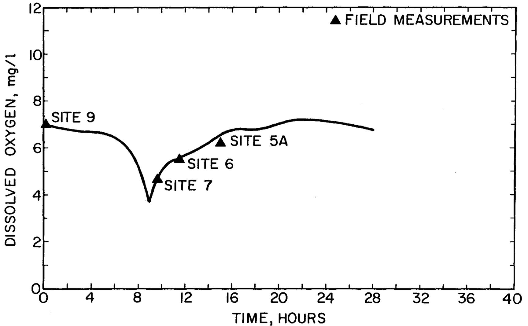
Figure 21. OXYGEN SAG CURVE FOR Q = 6 cfs AND TIME OF TRAVEL BASED UPON AVERAGE VELOCITY.
