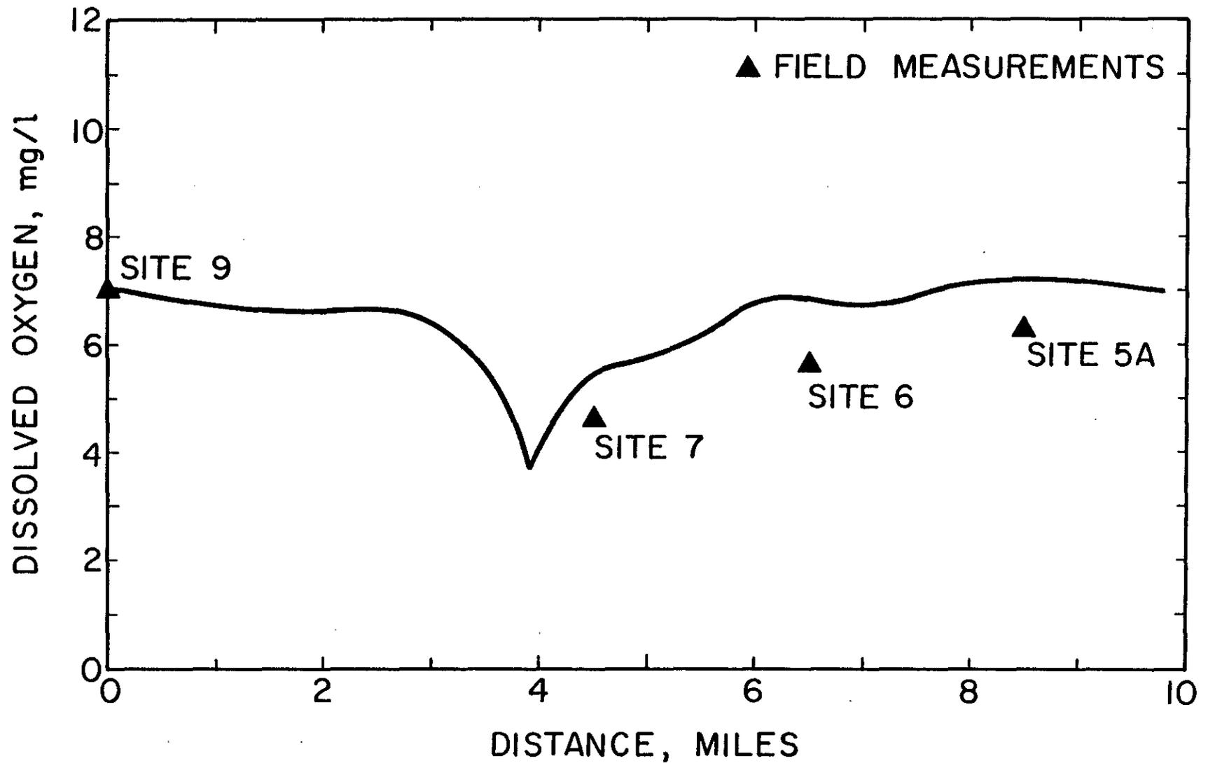
Figure 24. OXYGEN SAG CURVE VS. DISTANCE FOR Q = 6cfs AND TIME OF TRAVEL BASED UPON AVERAGE VELOCITY.
