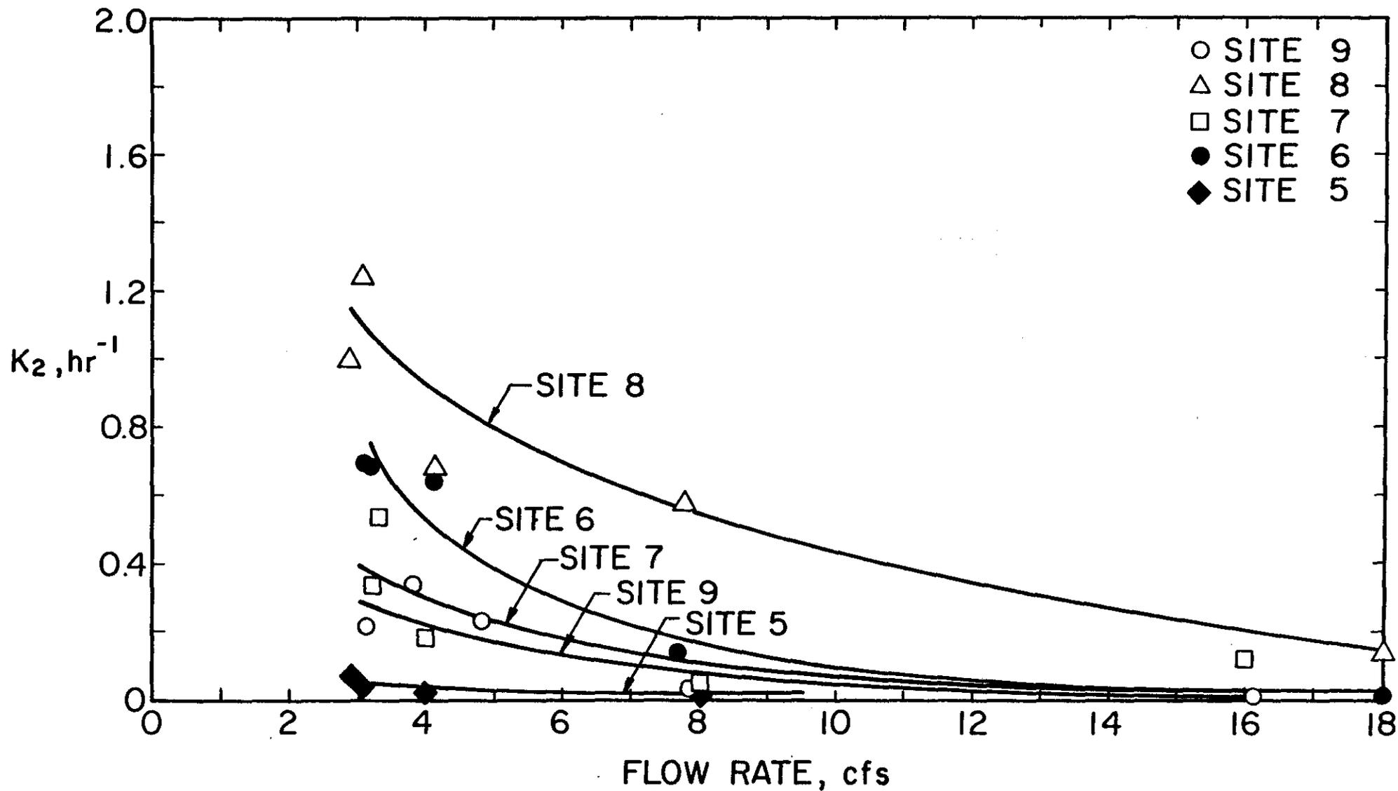
Figure 12.  $K_2$  AS A FUNCTION OF FLOW RATE FOR BLACK BEAR CREEK.<sup>43</sup>
