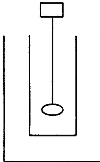
Figure 2. OPEN JAR REACTOR.
