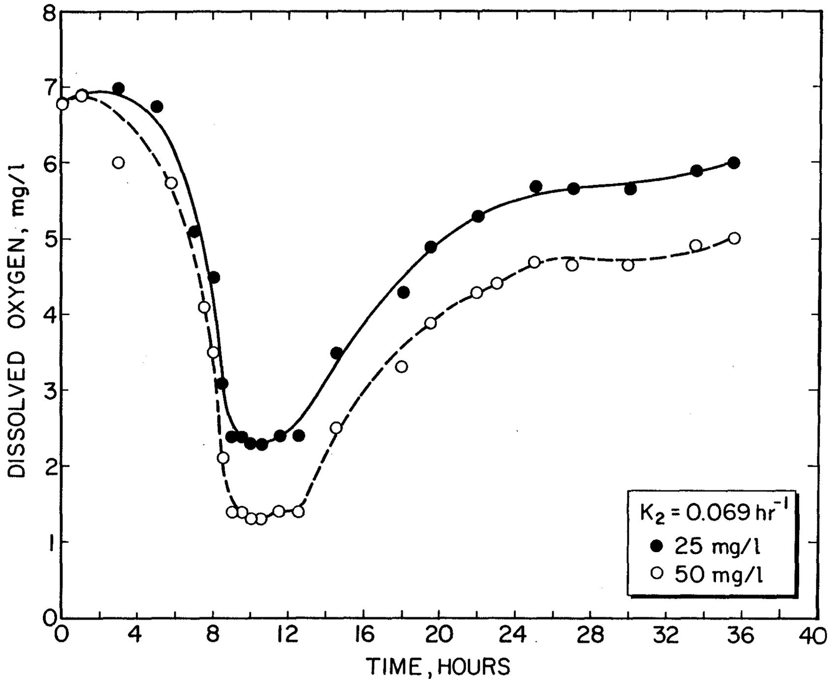
Figure 15. DISSOLVED OXYGEN PROFILES FOR  $S_i = 25 \text{ mg/l}$  AND  $S_i = 50 \text{ mg/l}$ .
