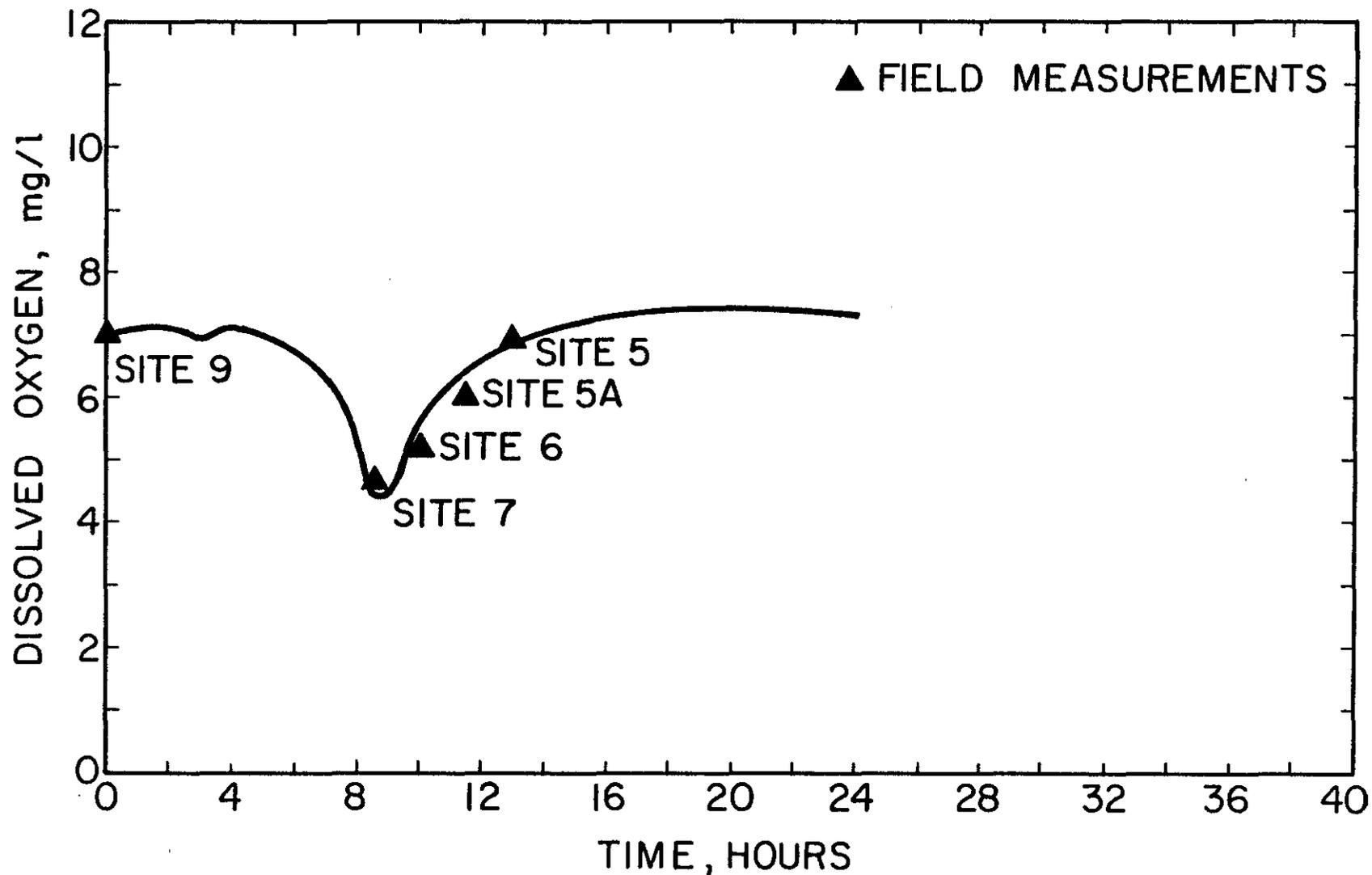
Figure 23. OXYGEN SAG CURVE FOR Q = 2.6 cfs AND TIME OF TRAVEL BASED UPON AVERAGE VELOCITY.
