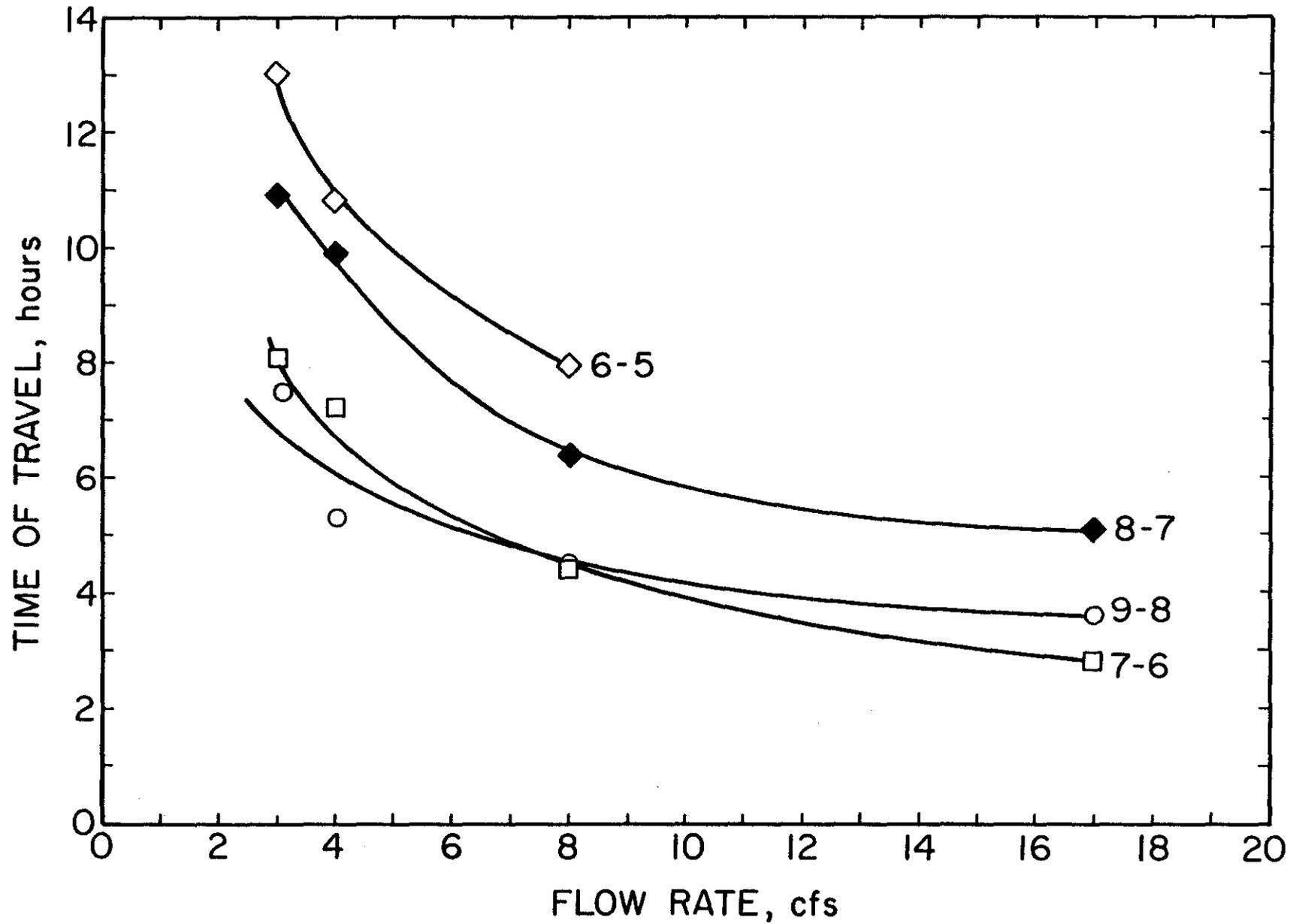
Figure 14. TIME OF TRAVEL AS A FUNCTION OF FLOW RATE. TIME OF TRAVEL BASED UPON MANNINGS EQUATION.
