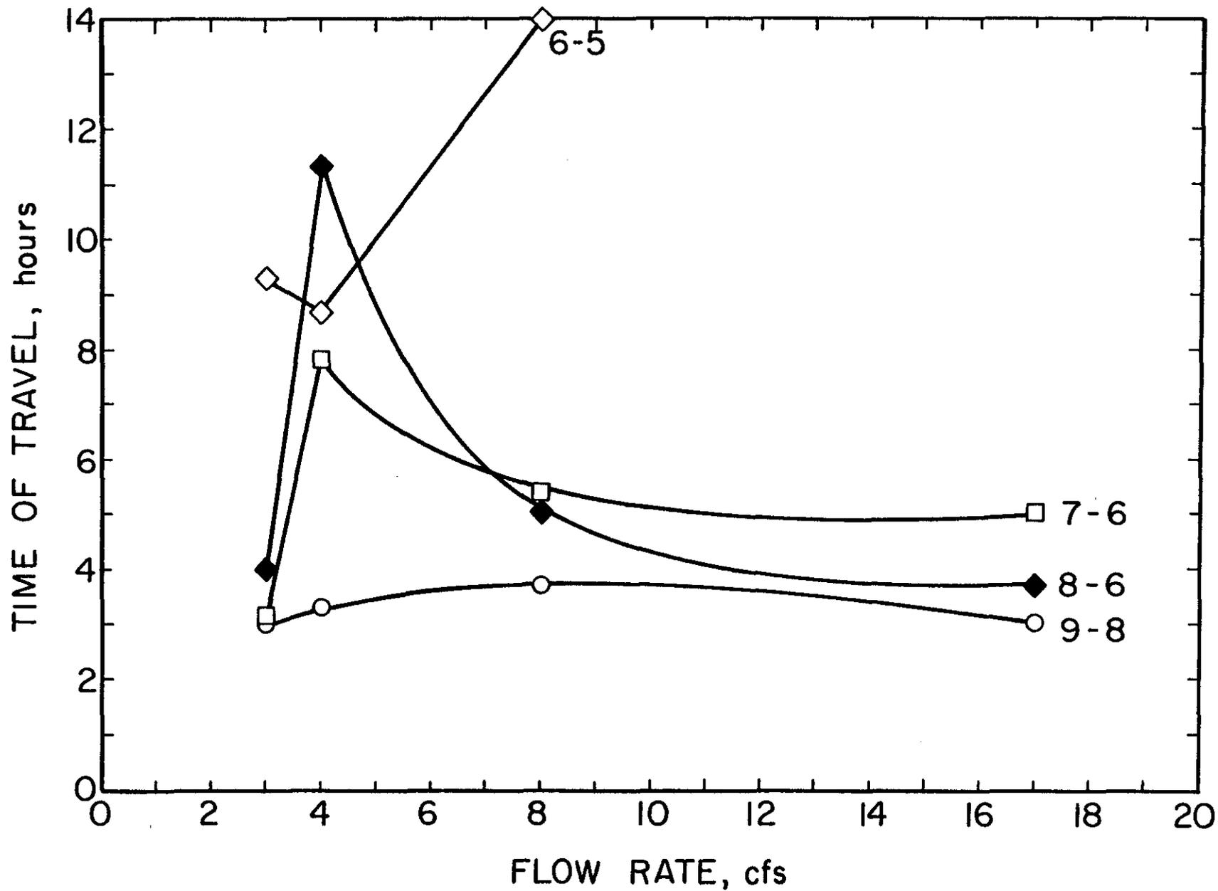
Figure 13. TIME OF TRAVEL AS A FUNCTION OF FLOW RATE. TIME OF TRAVEL BASED UPON AVERAGE VELOCITY.
