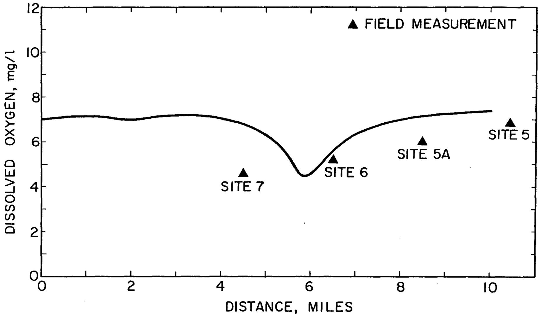
Figure 25. OXYGEN SAG CURVE VS. DISTANCE FOR  $Q = 2.6$  cfs AND TIME OF TRAVEL BASED UPON AVERAGE VELOCITY.
