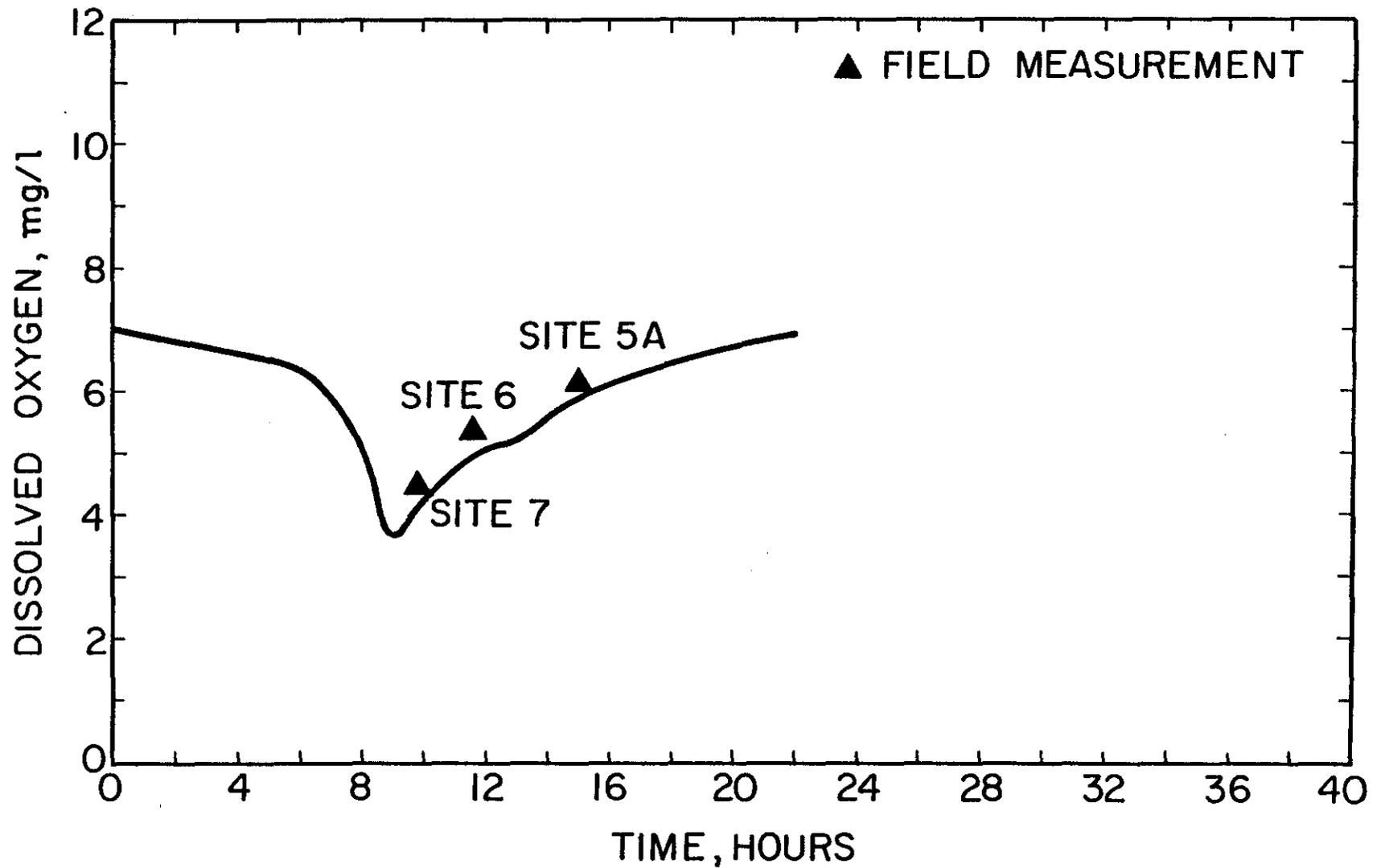
Figure 26. OXYGEN SAG CURVE FOR Q = 6 cfs AND TIME OF TRAVEL BASED UPON OXYGEN SAG.
