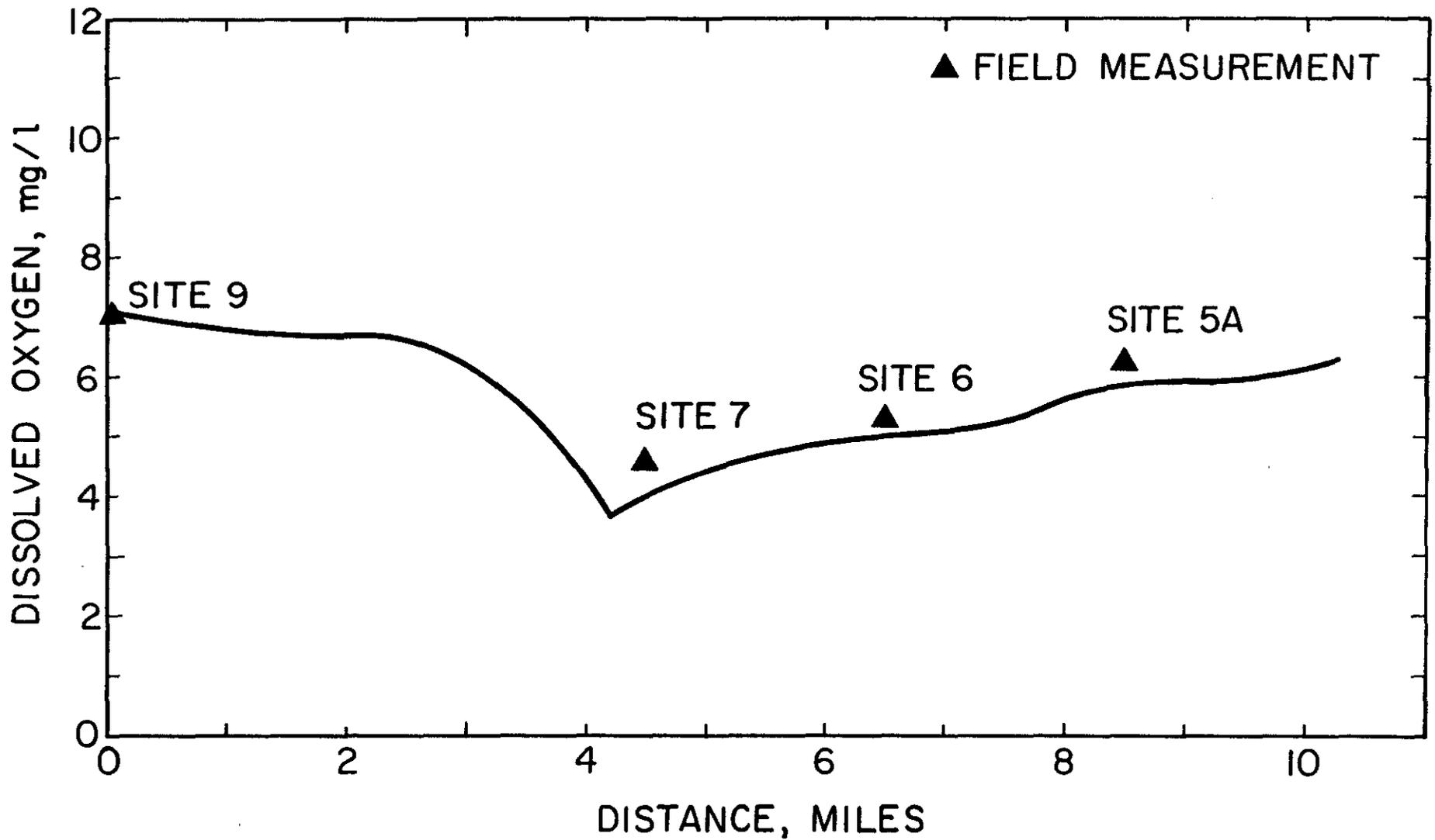
Figure 27. OXYGEN SAG CURVE VS. DISTANCE FOR Q = 6 cfs AND TIME OF TRAVEL BASED UPON OXYGEN SAG.
