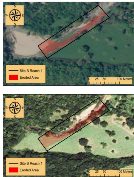
Figure 10. NAIP aerial images from 2003 (bottom) and 2008 (top) of a stream and the polygon (in red) showing the area of bank eroded during that time period.
