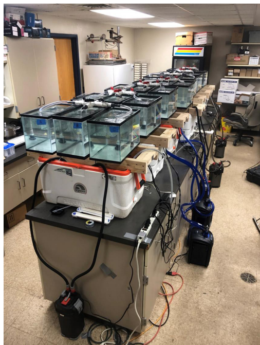
Figure 1. Image of tank setup showing seven treatment levels (cooler/tank complex) and three replicates (A, B, and C).
