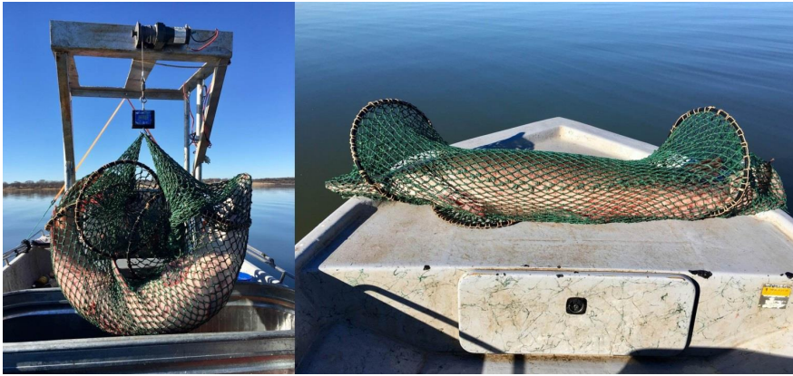
Figure 1. Photographs depicting the winching apparatus used to weigh Alligator Gar and the fish sock (25.4 mm #60 green-twine mesh x 3.05 m long x 457.2 mm diameter) used to support Alligator Gar.
