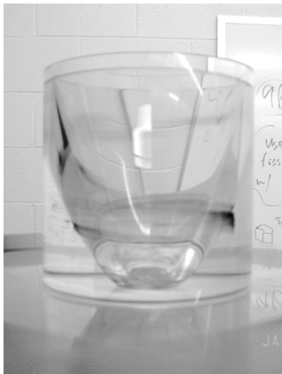
Figure 1. Green food coloring employed as a flow visualization aid. The food coloring trace emulates the qualitative features of the fluid motion apart from the change of elevation of the dye.
