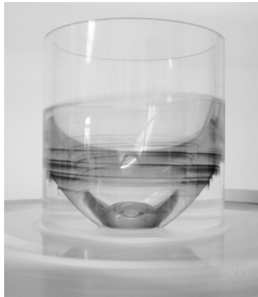
Figure 2. Crystal Violet employed as a flow visualization aid. Stain shows some departure from actual fluid motion
