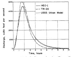
FIGURE 2. Unit hydrographs for Deep Fork Creek at Eastern Avenue
