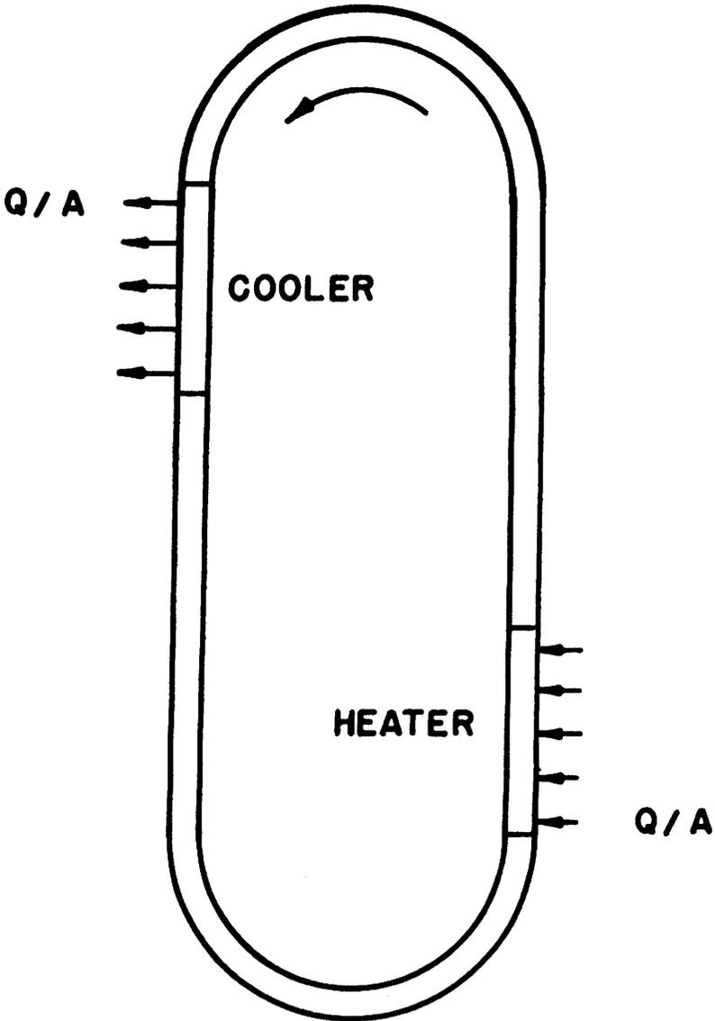
Figure 1. Natural-circulation loop schema
