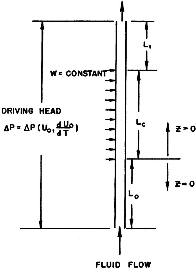
Figure 3. Idealized schema of the natural-circulation loop
