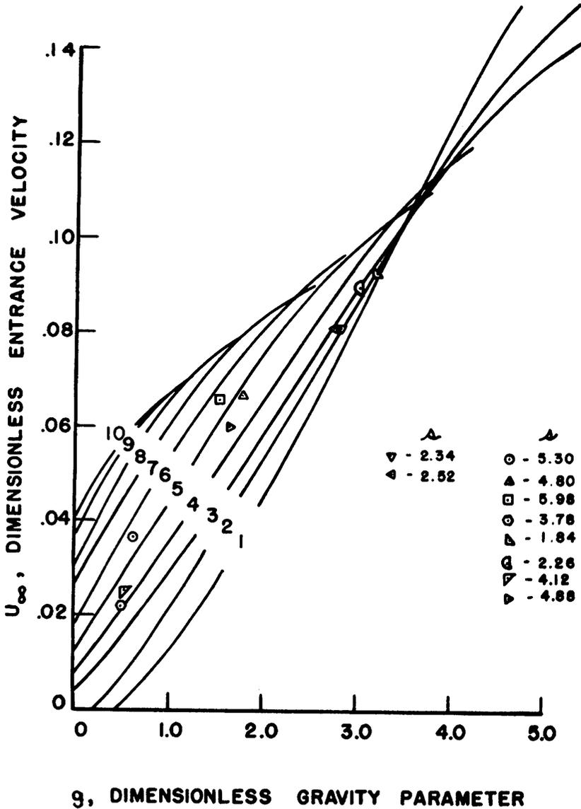
Figure 6. Results with Freon-12 and Freon-114 at various subcooling
