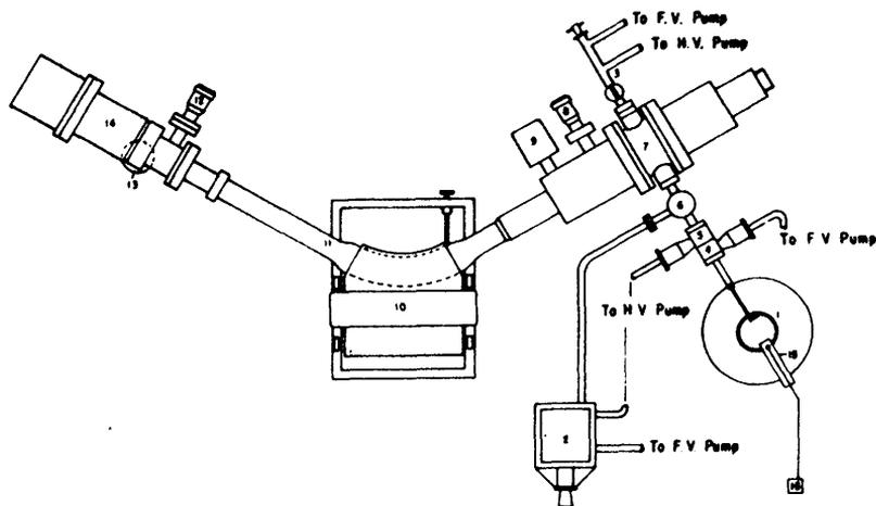
Figure 3. Drawing of analyzer unit showing vacuum connections. Numbers are the same as in Figure 1.
