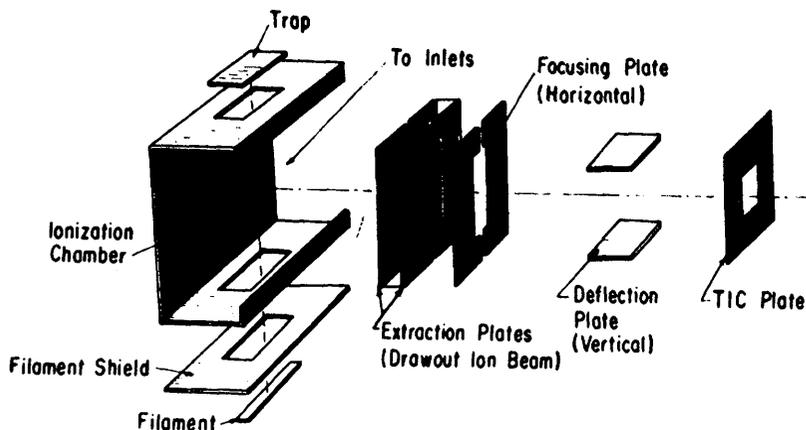
Figure 6. Schematic of ion source.
