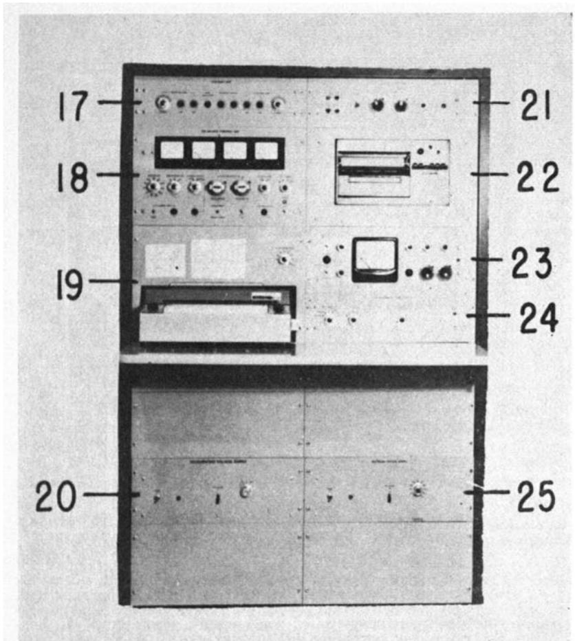
Figure 5. Front view of control unit. 17. Ion beam focusing controls. 18. Ion source controls. 19. Pen and ink recorder for monitoring total ionization current. 20. Acceleration voltage supply. 21. Gas chromatography peak splitting unit. 22. Oscillographic recorder. 23. Magnet power control unit. 24. Galvanometer amplifier. 25. Electron multiplier voltage supply.
