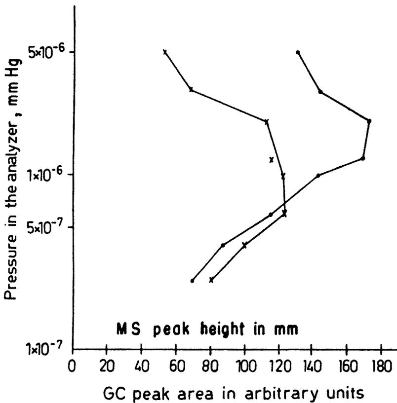
Figure 15. Pressure in the analyzer as a function of GLC peak areas and the mass spectrum peak height (from Ryhage, 1967).
