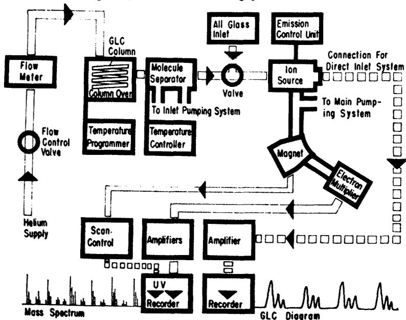
Figure 1. Block diagram of the Oklahoma State University mass spectrometer-gas chromatograph.
