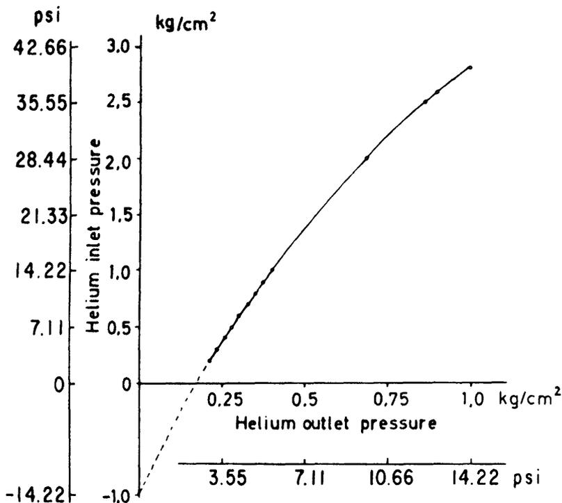
Figure 13. Helium pressure at the outlet as a function of the helium inlet pressure of the GLC column when connected to the separator (from Ryhage, 1967). The same GLC column was used as in Figure 12.
