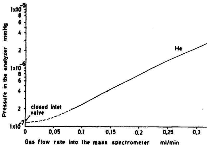
Figure 11. Pressure in the analyzer as a function of the gas flow into the mass spectrometer for helium (from Ryhage, 1967).
