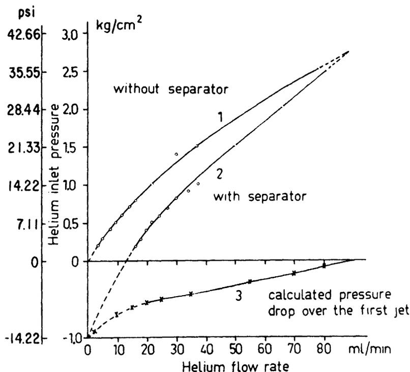
Figure 12. Helium inlet pressure as a function of the helium flow rate at the column outlet (from Ryhage, 1967). The GLC column used was 3 mm  $\times$  2 m and packed with 2% SE-30 on silanized Gas Chrom P, 30-100 mesh. The separator dimensions in mm are:  $d_1 = 0.1$ ,  $d_2 = 0.4$ ,  $d_3 = 0.25$ ,  $d_4 = 0.4$ ,  $l_1 = 0.1$ , and  $l_2 = 0.2$  (Fig. 8). Column temperature 200 C.
