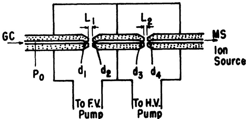
Figure 8. Schematic of molecule separators.
