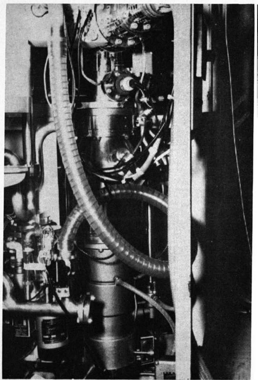
Figure 7. View of oil diffusion pump.
