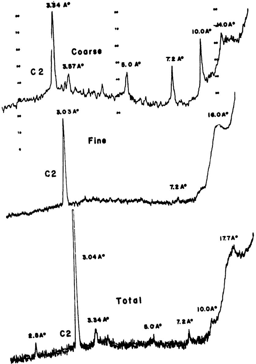
Fig. 3. X-ray Spectrographs of Waurika No. 1 C2 Horizon Showing Coarse, Fine, and Total Clay
