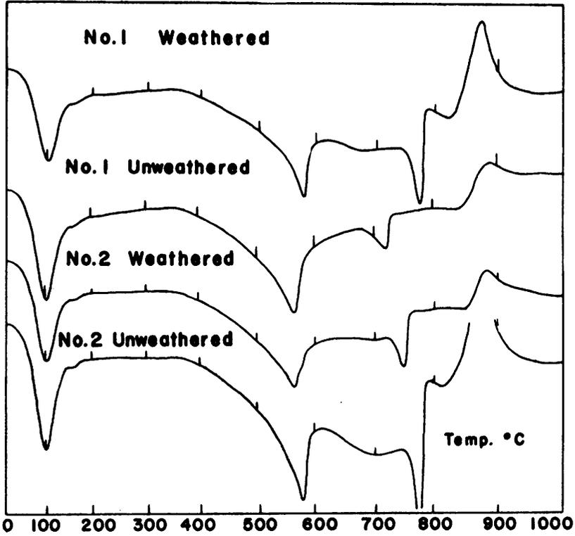
Fig. 2. Differential Thermal Curves for Total Clay of Wellington Formation Samples
