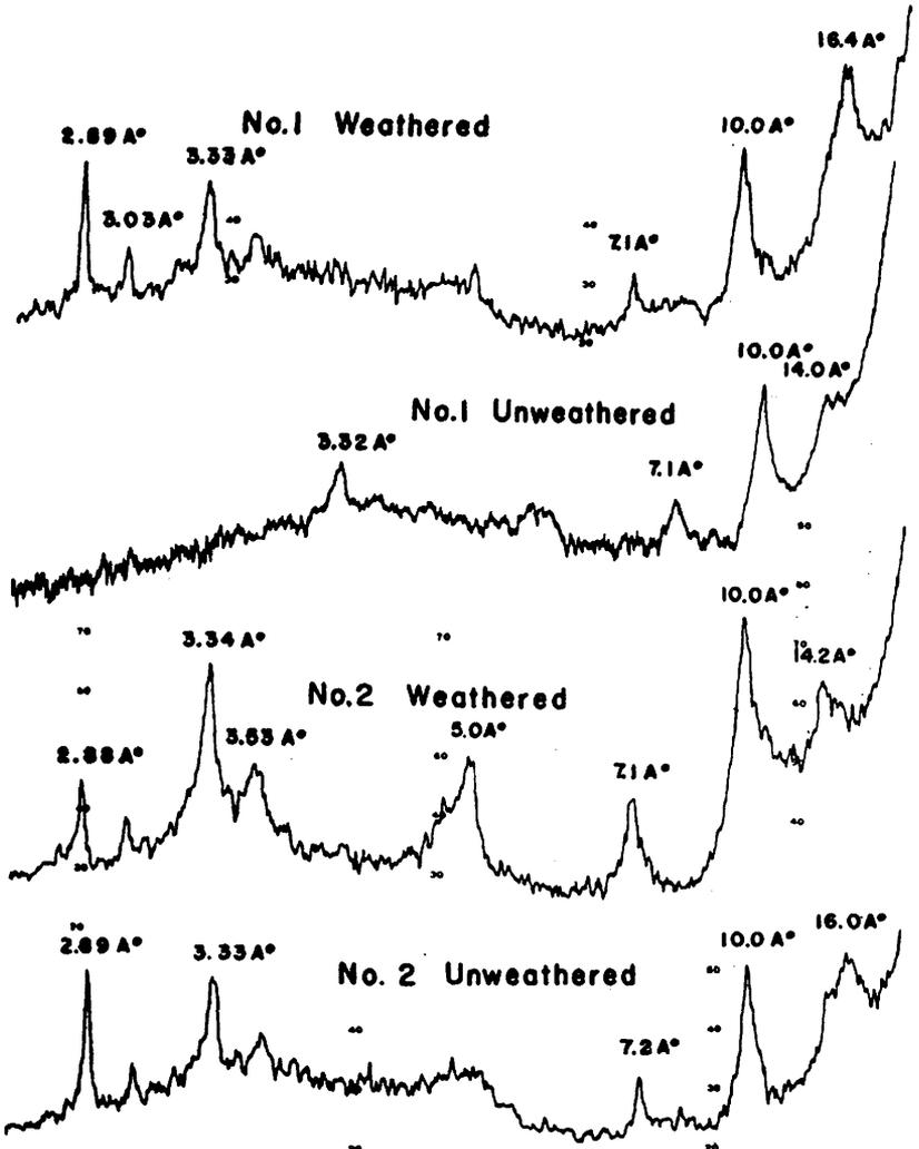
Fig. 1. Total Clay X-ray Spectrographs of Wellington Formations Samples
