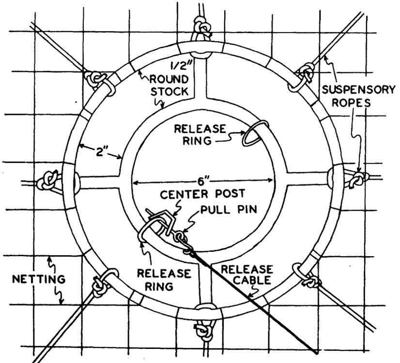
Figure 2. Drop-net trap, assembly detail Center Ring Assembly.
