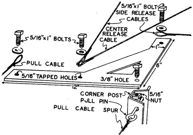
Figure 3. Drop-net trap, assembly detail
