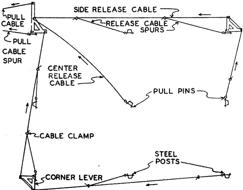
Figure 4. Drop-net trap, assembly detail.
