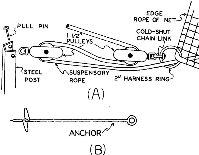
Figure 1. Drop-net trap, assembly detail
