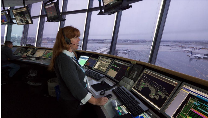
Figure 1. Ramp controller station, including ramp controller view of the ramp area and computer displays of gate areas and aircraft arrival/departure timeline. Adapted from “EWR Ramp Controller” n.d. Reprinted with permission.
