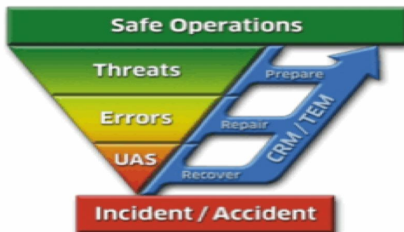
Figure 1: Threat and Error Management Model (Adapted from United Airlines)
